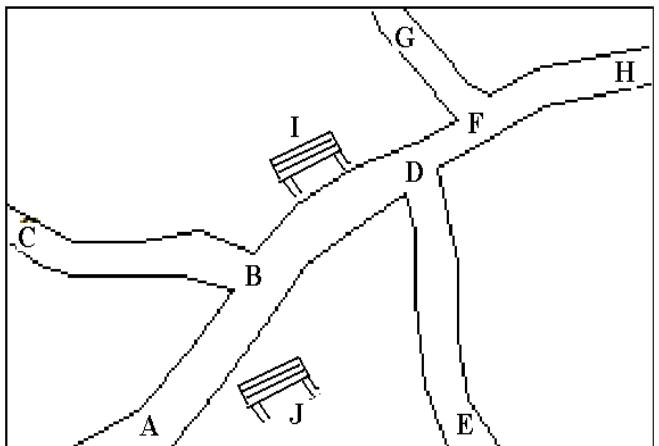
Fig. (3). Topographical representation of environment. Entry/exit zones (A, C, E, G, H), junctions (B, D, F), stop zones (I, J), paths (AB, CB, BD, DF, etc) and routes (ABDFH, ABC, EDFG, etc) are depicted.
