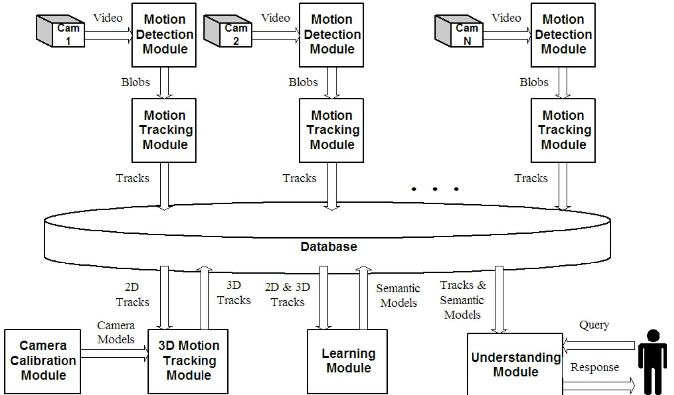
**Fig. (1).** Architecture of the KUES system.
