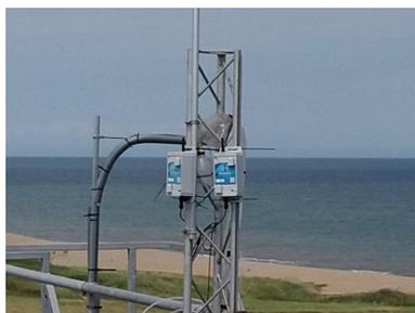
**Figure 1.** View of the co-located equipment at WAO: cost-effective devices 5158 and 5178 are the two blue and grey boxes.
