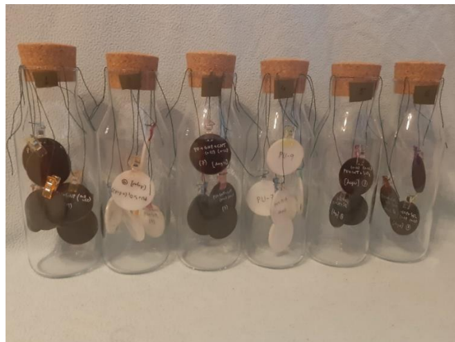
Figure 6.4. The specimens inside glass bottles for the water absorption test at 32 °C and 45 °C.
