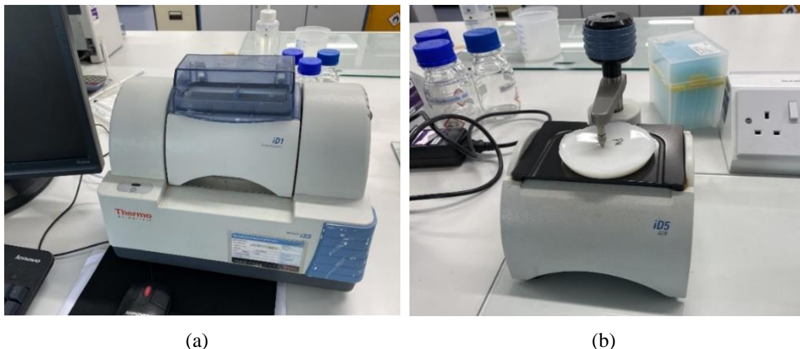
Figure 4.7. (a) Thermo Nicolet iS5 FTIR spectrometer, and (b) iD5 Diamond ATR accessory
