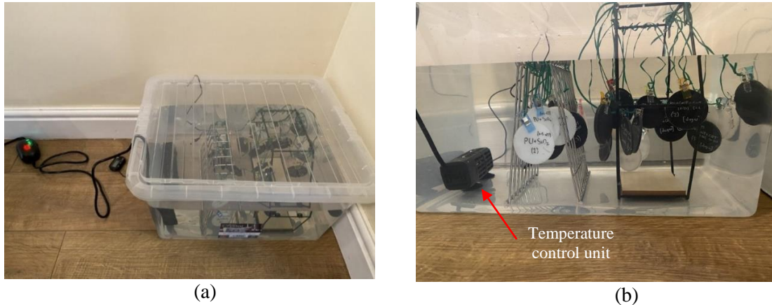
Figure 6.3. (a) Specimens submerged in water at RT in a plastic container, (b) Close-up view showing the temperature control unit.
