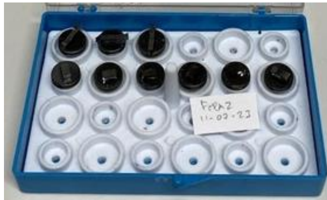
Figure 5.4. Specimens mounted on stubs for SEM imaging.
