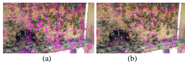
Figure 5 : (a) Segmentation of bees with bounding rectangles in an image, (b) the same image, but with a restriction applied on the width to length ratio of the rectangles.
