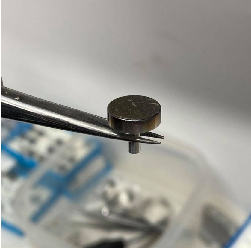
Figure 6: An image showing one of the aluminium carbon coated stubs which are placed inside the SEM and used in all three experiments.
