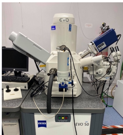
Figure 9: An image showing the Zeiss Evo 50 SEM with associated Oxford Instruments Inca Analytical Suite utilising X-Act EDS Detector used in all three experiments, based at Kingston University.
