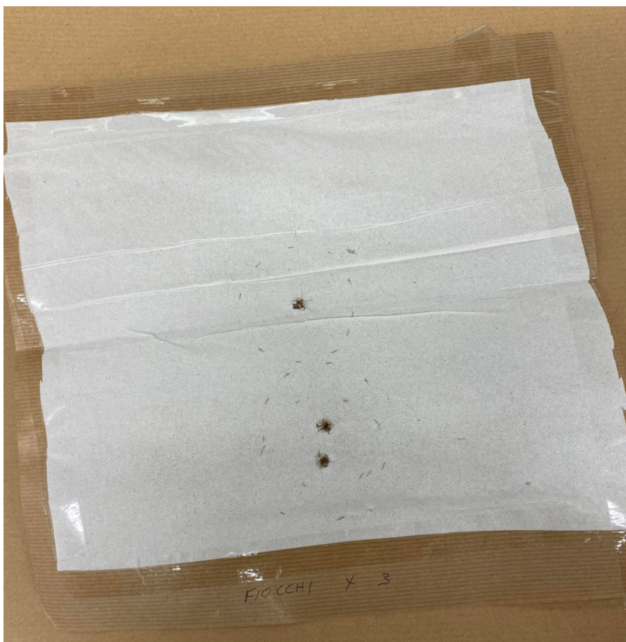
Figure 17: Photograph showing a target after three rounds of Fiocchi ammunition were fired directly at said target, sent to Kingston University by the Garda Siochana.
