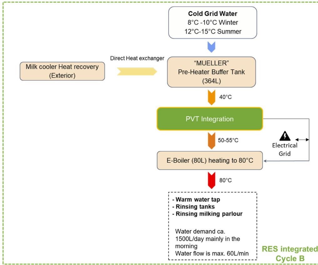
Fig. 5. Overview of the proposed system with PVT collectors at the LVAT-ATB dairy farm in Germany.
