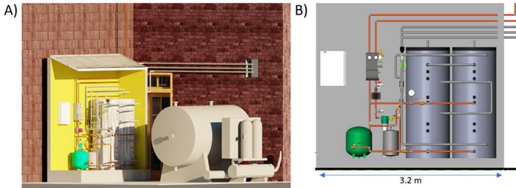
Fig. 18. Placement of the solar station house, B) Component placement inside the solar station house.
