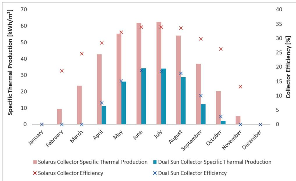
Fig. 8. Collector efficiency and specific thermal production at the LVAT-ATB dairy farm in Germany.
