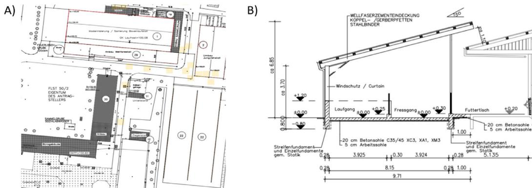
Fig. 15. A) plan of farm B) roof layout of building B29.
