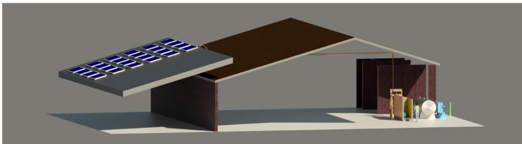
Fig. 12. Locations of PVTs, solar station, and technical room in LVAT-ATB dairy farm.
