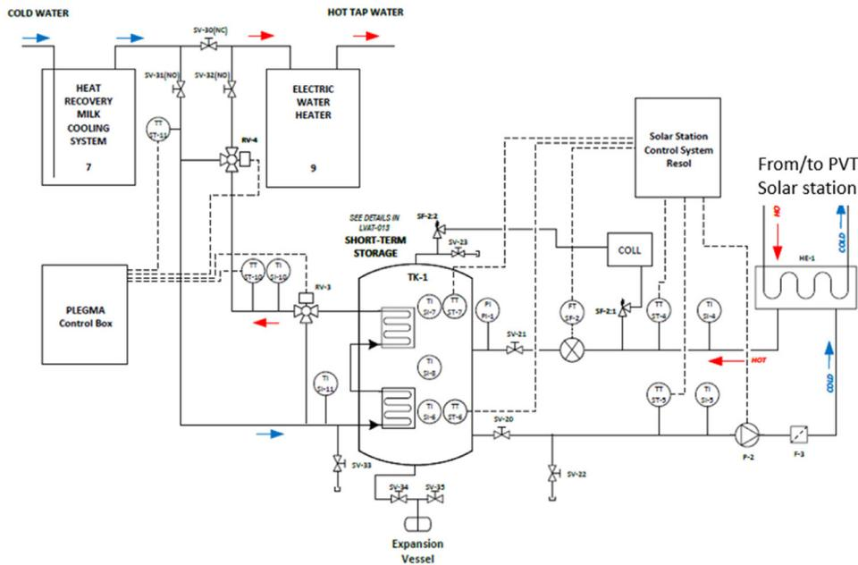
Fig. 16. First P&ID design of PVT system at LVAT-ATB dairy farm in Germany.
