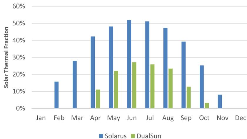
Fig. 11. Monthly solar fraction values for Solarus and DualSun PVT collectors at the LVAT-ATB.
