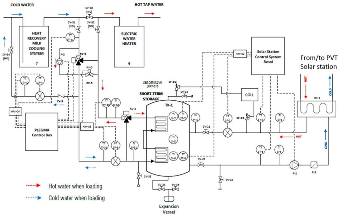
Fig. 17. Second P&ID design of PVT system at LVAT-ATB dairy farm in Germany.
