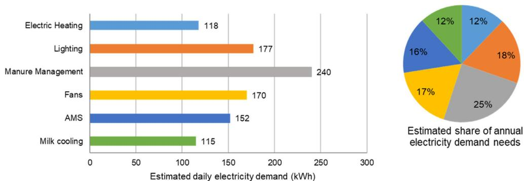
Fig. 4. Estimated daily electricity demand breakdown (left) and percentage of annual electricity demand (right) at LVAT-ATB in Germany.
