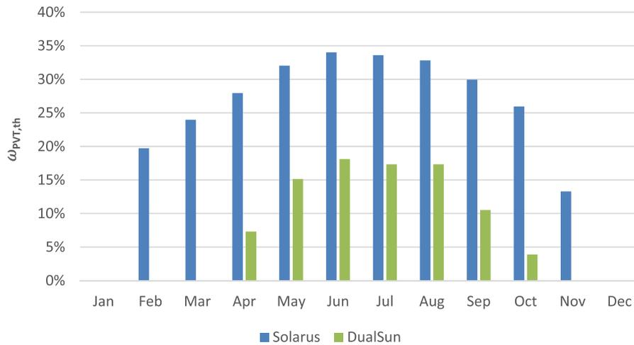
Fig. 10. Monthly thermal energy utilization ratio for Solarus and DualSun PVT collectors at the LVAT-ATB.
