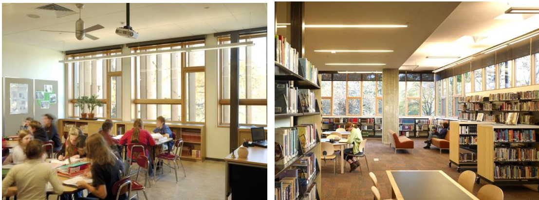
Figure A29 Abundant use of daylight in library (left and right); artificial illumination is controlled by sensors (right) (Kieran Timberlake Architects, 2010; AIA, 2020)
