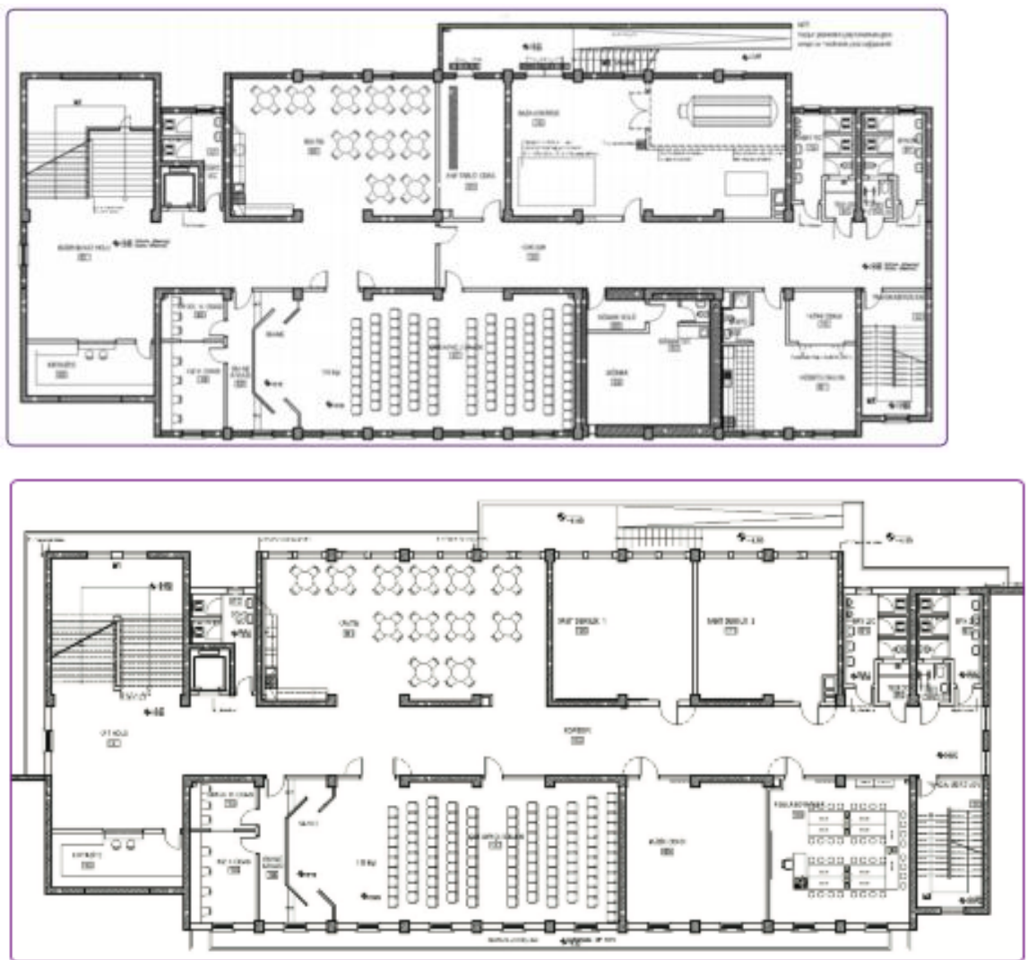
Figure 2.10 An example from a standard (10025R-480 code) K-12 school's floor plan (above) and revised floor plan (below) (Kose and Barkul, 2012)
