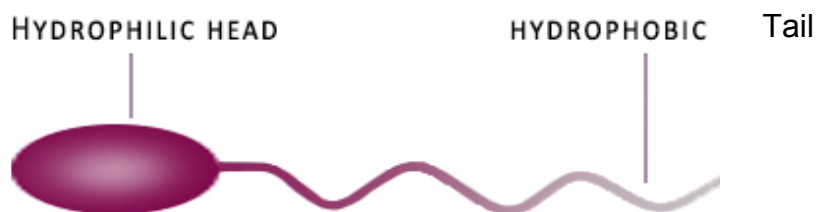
Figure 1.8: Schematic structure of surfactants. Showing a hydrophilic head made of polar chemical group and hydrophobic tail made of aliphatic hydrocarbon chain (92).
