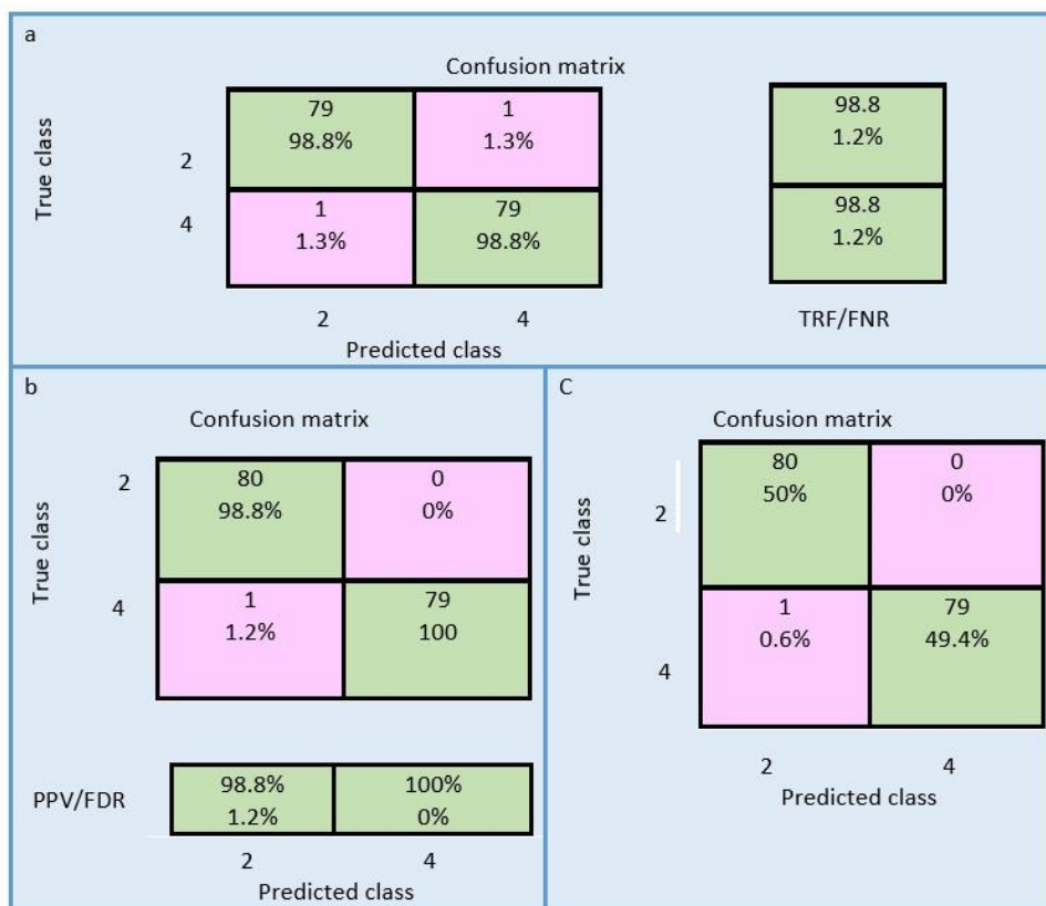
Figure 33: Presents confusion matrix for boosted tree classification with Ada boost ensemble method and 200 learners.
