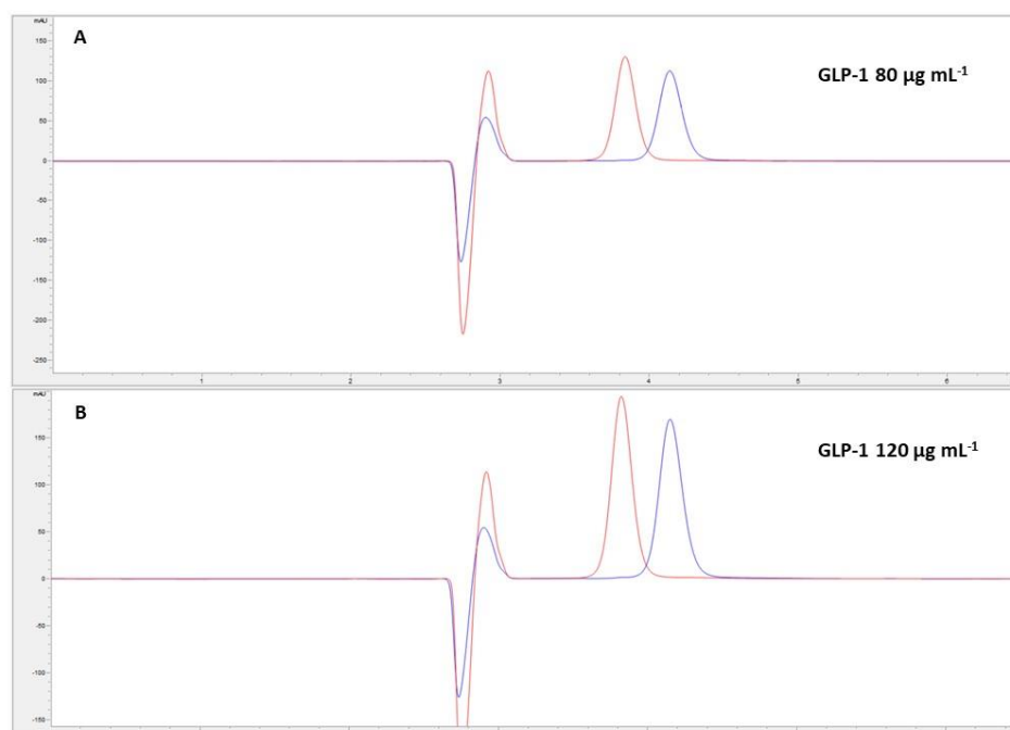
Figure 58: HPLC chromatograms for GLP-1 dissolved in distilled water (GLP-1 concentration A: 80 \mu\text{g mL}^{-1} and B: 120 \mu\text{g mL}^{-1} ) with two different compositions of mobile phase A: acetonitrile with 0.1% TFA (red) or acetonitrile alone (blue). (Area and height: t-test, p > 0.05 ). Vertical axis represents area (mAU), and horizontal axis represents retention time (min).
