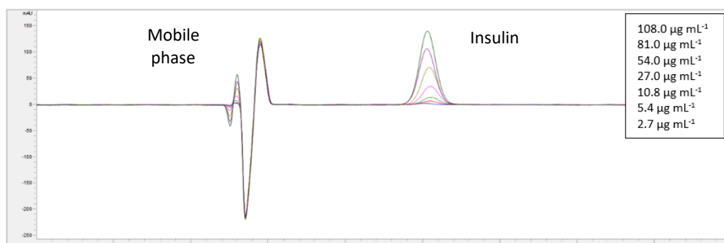
Figure 31: HPLC chromatograms for the calibration curve of human insulin in the concentration range from 2.7 \mu\text{g mL}^{-1} (bottom) to 108.0 \mu\text{g mL}^{-1} (top). Average retention time: 5.07 \text{ mins} \pm 0.03 \text{ mins} , asymmetry factor: 1.00 \pm 0.02 , tailing factor: 1.00 \pm 0.02 , and efficiency of chromatography peak: 2392.91.
