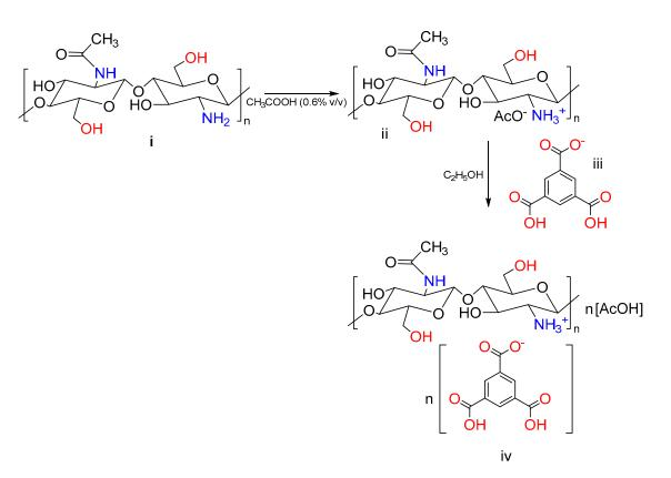
**Figure 4.** Schematic representation of the cross-linking effect of BTC in the formation of chitosan hydrogels: (i) chitosan; (ii) protonated chitosan; (iii) BTC; and (iv) chitosan glucosamine carboxylate salt.
