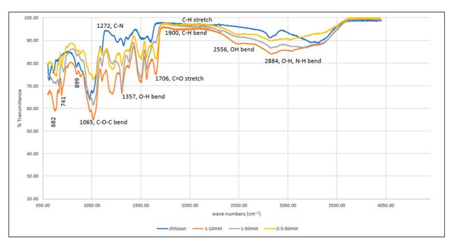
Figure 7. FTIR spectrum of uncross-linked and cross-linked chitosan hydrogel (in different concentrations).
