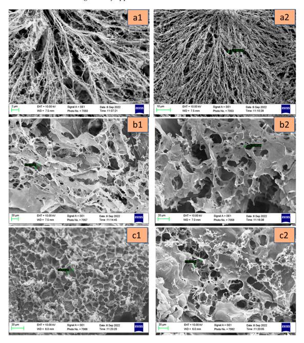
**Figure 11.** SEM structures of freeze-dried chitosan hydrogels M1 (**a1**,**a2**), M2 (**b1**,**b2**), and M3 (**c1**,**c2**) at different magnifications.
