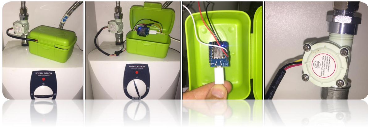
Figure 5.4: The self-made Arduino-Uno based immersion heater inspector consists of a YF-S201 water flow sensor and Wi-Fi- and Bluetooth-Modul NodeMCU ESP32
