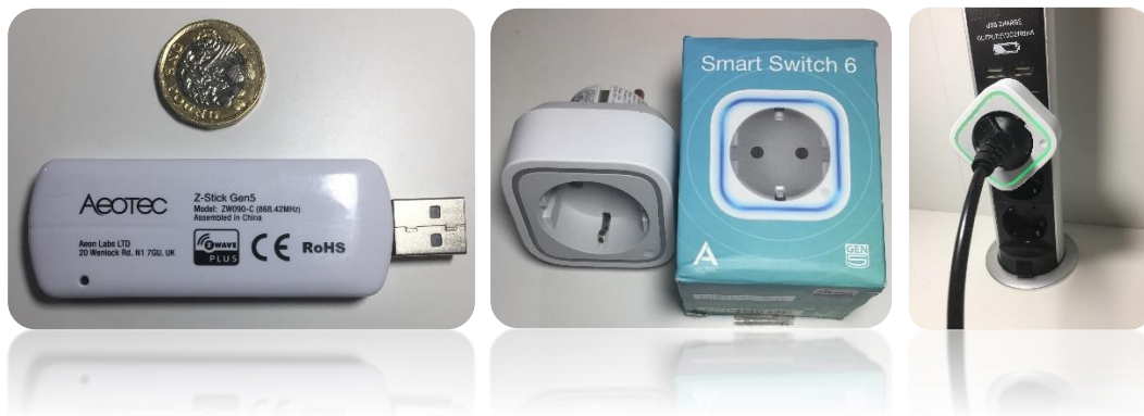
Figure 5.1: ZW-ECR Module mainly consists of a Z-Stick GEN5 controller, smart switch 6 from AEON-LABS
