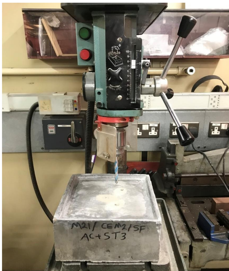
Figure 3.15 Drilling device used to obtain powdered samples
