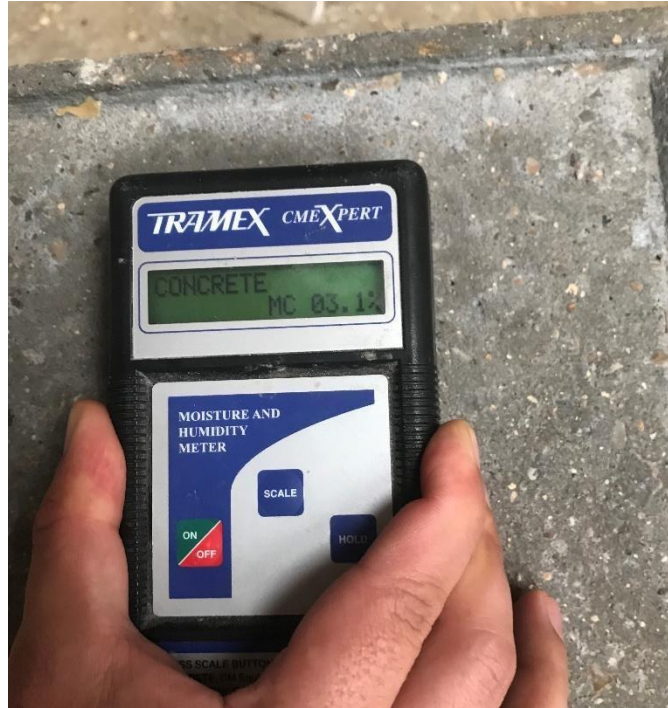
Figure 3.2 Moisture content measurement of specimens
