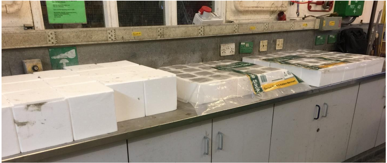
Figure 3.5 Casting concrete in polystyrene moulds
