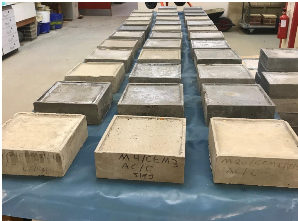
Figure 3.12 Slabs after air and water curing
