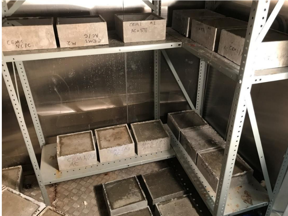
Figure 3.13 Slabs placed in freeze-thaw chamber
