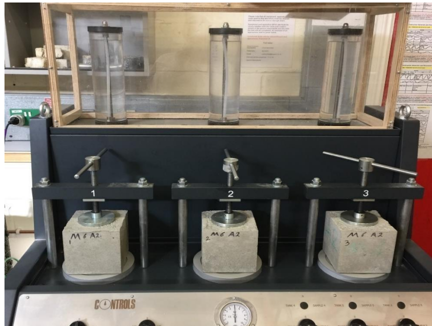
Figure 5.24 Water permeability under pressure apparatus
