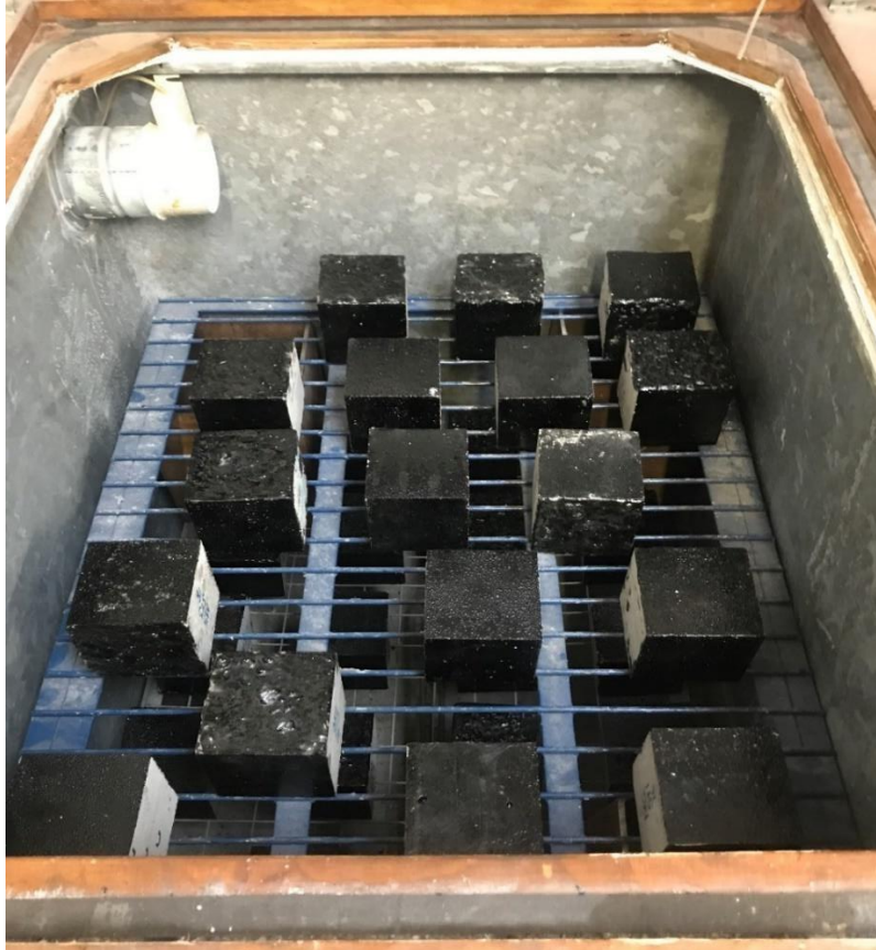
Figure 3.11 Carbonation chamber apparatus
