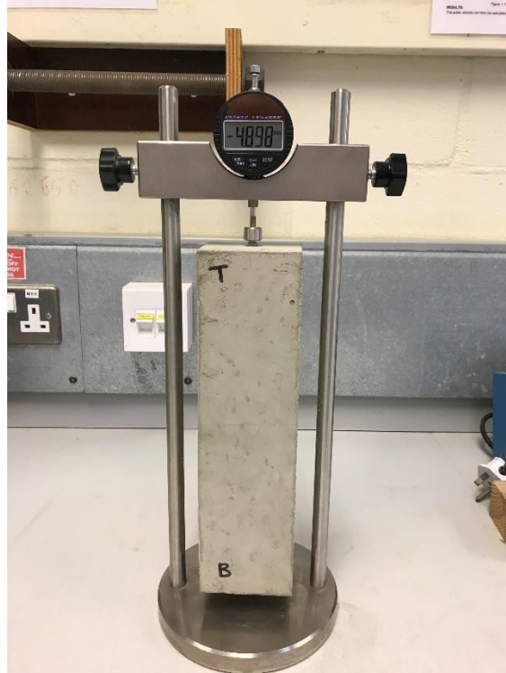
Figure 3.7 Drying shrinkage comparator
