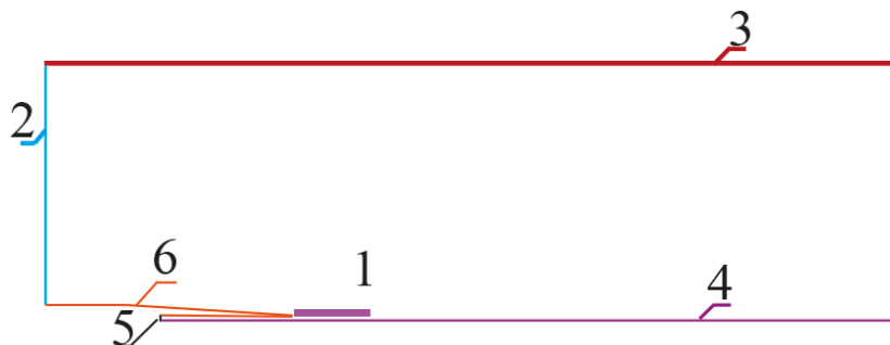
Figure 3: Geometry to study gas dynamics of propane-air flame in case of plasma domain (1). Boundary conditions include inlet and exterior flux of air (2), outlet (3), centreline (4), inlet of fuel mixture (5), wall condition for initiator (6).
