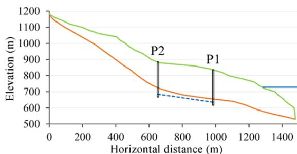
**Fig. 8** Cross-section through the western side of the landslide that includes piezometers P1 and P2. Water levels recorded around November 1961 (Müller 1964) are indicated by the ‘lower aquifer’ (Semenza 2001, 2010) water table (broken blue line) between the piezometers. The design top water level of the reservoir (722.5 m) is shown. From Dykes and Bromhead (2018a).
