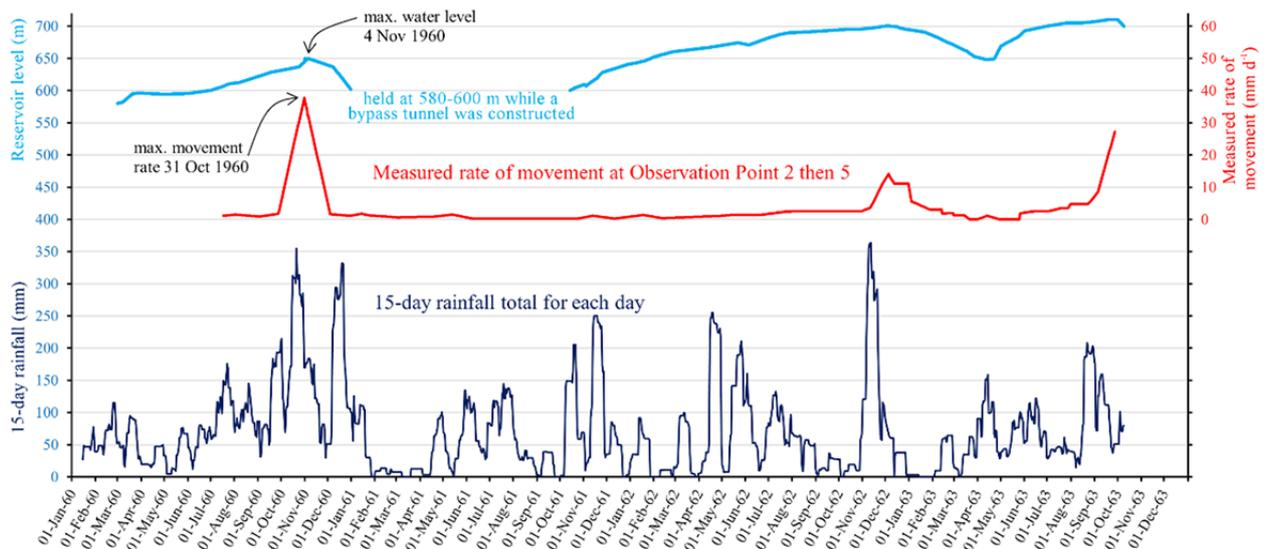
**Fig. 9** Composite graph of 15-day rainfall totals at Erto, reservoir water level elevation and movement rates in the lower western part of the developing landslide for the period 15 January 1960 to 9 October 1963 inclusive. From Dykes and Bromhead (2018a) partly after Müller (1964).
