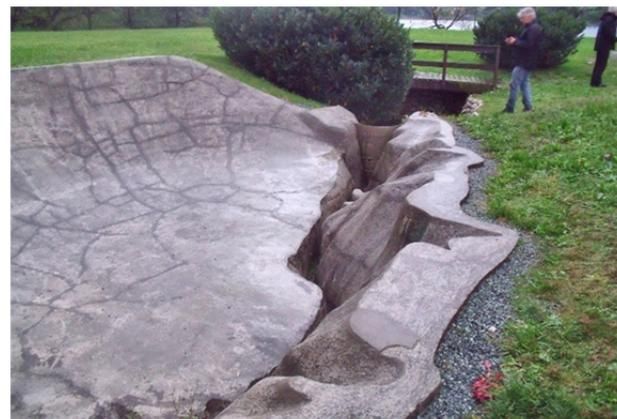
**Fig. 11** The 1: 200 scale model of the Vaiont landslide at Nove power station in 2013, showing the large sub-horizontal failure surface forming the assumed ‘chair’ shape. Photo: APD.
