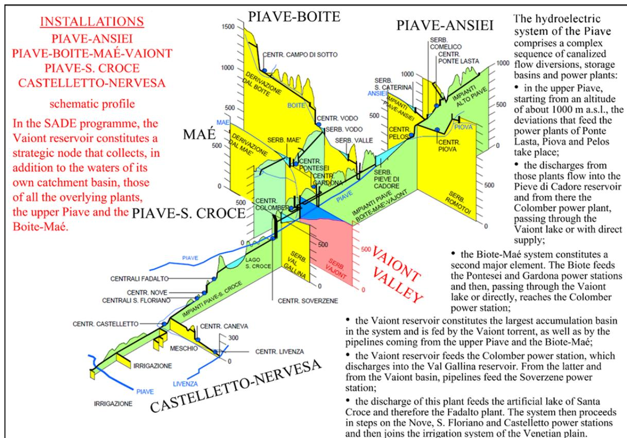
Fig. 3 Diagram showing the various elements of the entire Piave valley hydro-electric project. Source: Friulian Dolomites Natural Park archive (with permission).
