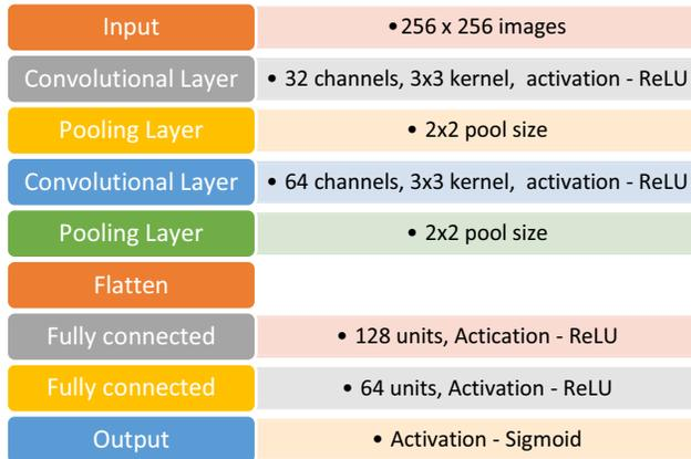
**Figure 2.** The CNN network architecture used for both sets of features.
