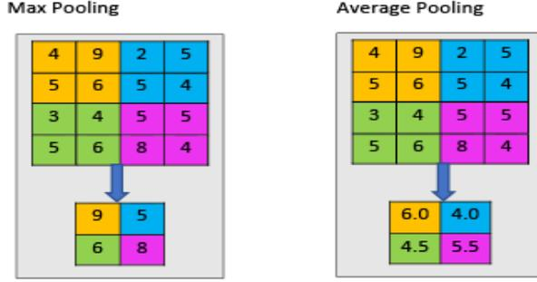
**Figure 1.** An illustration of the two most commonly used pooling methods with  $L = 2$  and  $S = 2$ .
