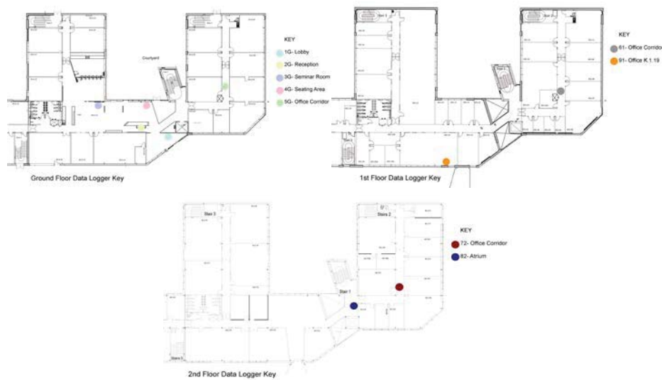
Figure 1. Floor plans of the case study building presenting the location of the data loggers
