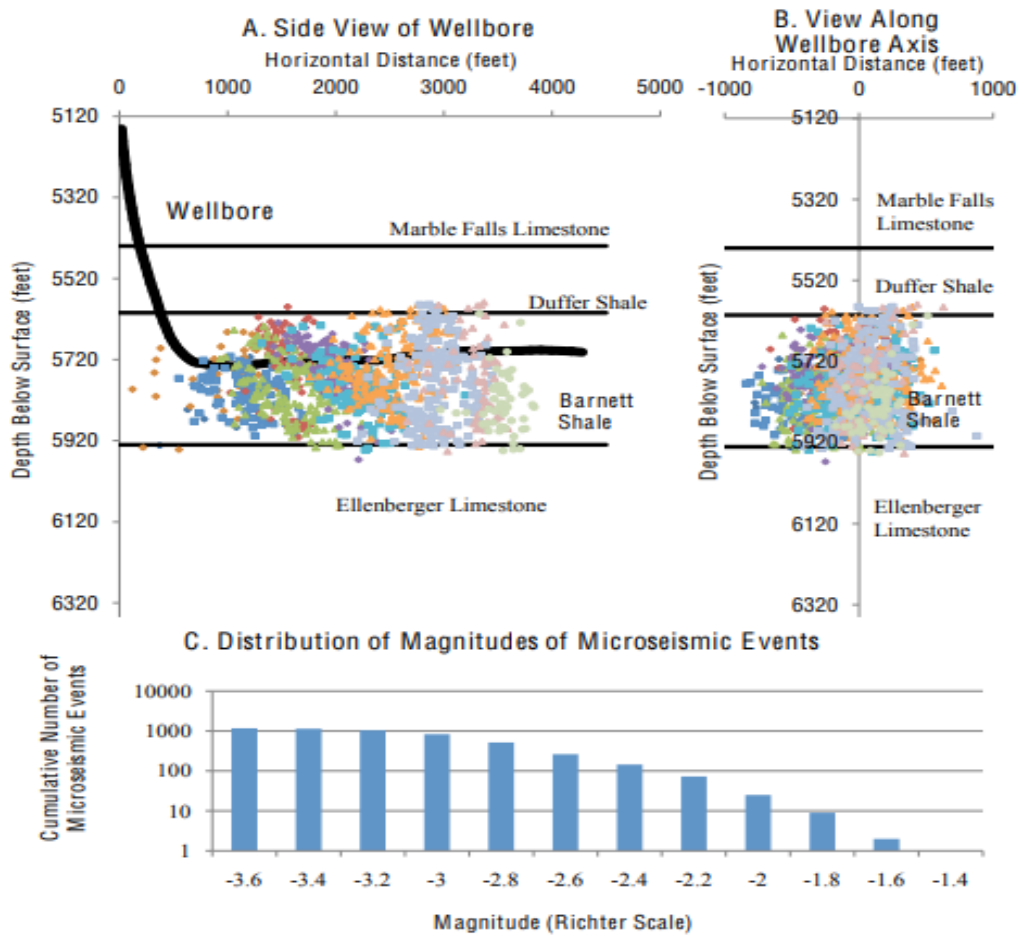
Figure 32. Microseismic Profile of Hydraulic Fracturing Operation in the Barnett Shale.
