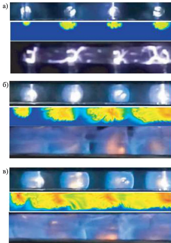
Fig. 1. Comparison of the results of experiments with spark ignition of the mixture (upper part of each fragment) with the results of modeling streamer ignition (middle part) and experiment with streamer ignition (lower part) in the case of eight ignition centers (half of the tube is shown) at times corresponding to (a) the occurrence of a discharge, (b) 3/400, and (c) 6/400 s.
