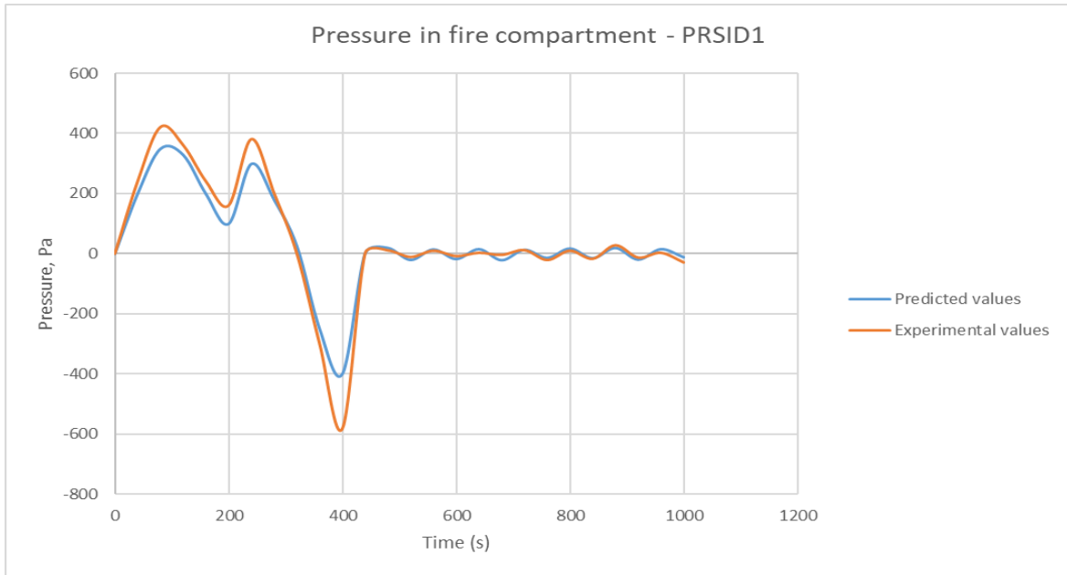
Fig. 7. Pressure variations inside the nuclear compartment -Predictions vs Experimental data (1000 first seconds of test-PRS_SI_D1).
