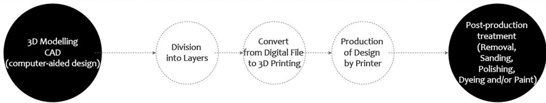
Figure 2 Standard stages of 3 D printing.
