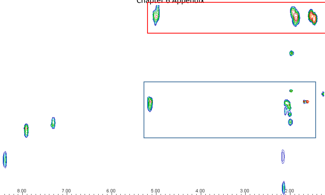
Figure 145 DOSY spectra, analysed in Dynamics centre highlighting the squalene peaks and proposed polymer peaks after 55 mins of UVC exposure on the sample
