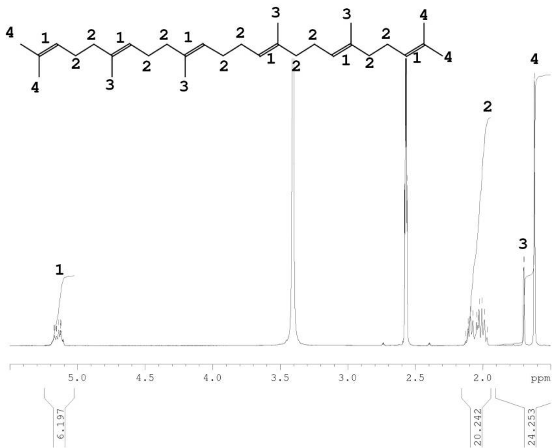
Figure 138 1D NMR spectra showing characterisation of Squalene 0.5% w/w; 256 scans, and same squalene concentration as polymerization experiment samples
