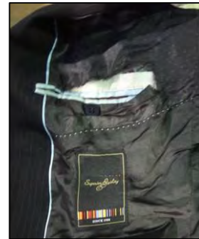
Figure 8. Jacket linings ripped at pocket seam.
