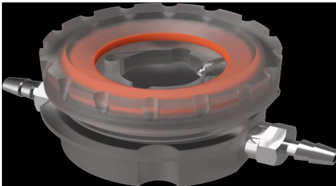
Figure 8.2 Flow cell apparatus. Can be set up under a microscope and input and output tubes for media flow can be inserted into both ends.
