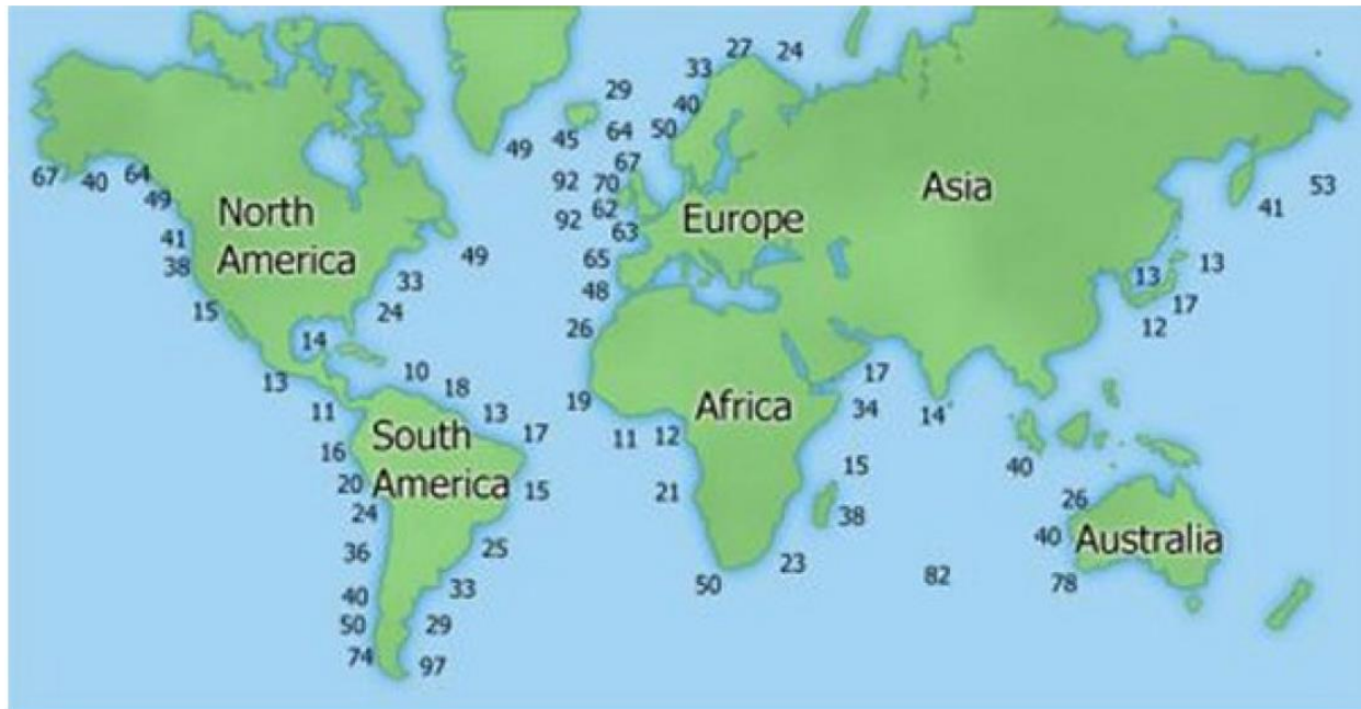
Figure 10 Wave energy potential worldwide (source: European Directory of Renewable Energy, 1991)
