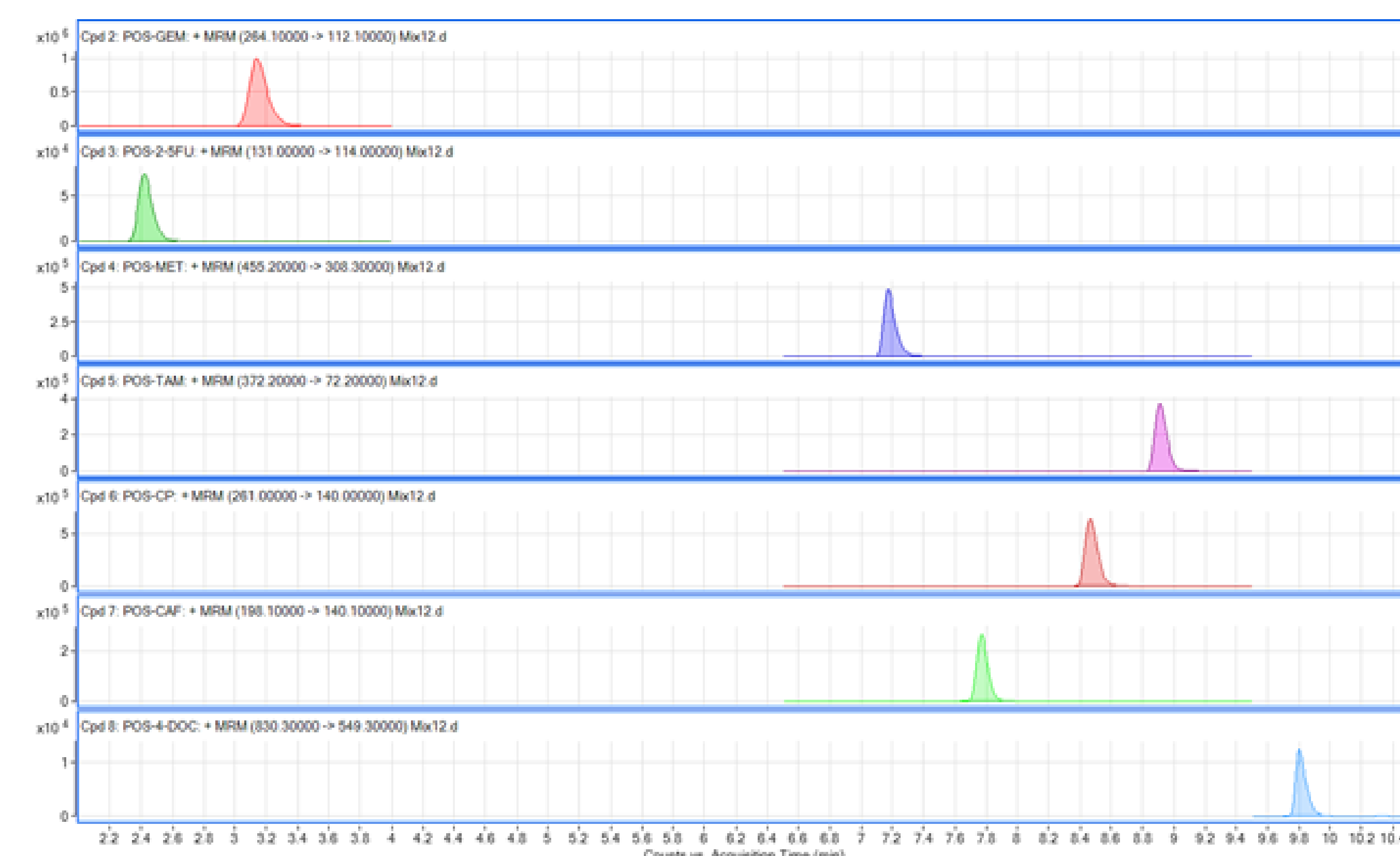
Figure 3: Chromatogram showing the separation of six anticancer drugs and the internal standard
