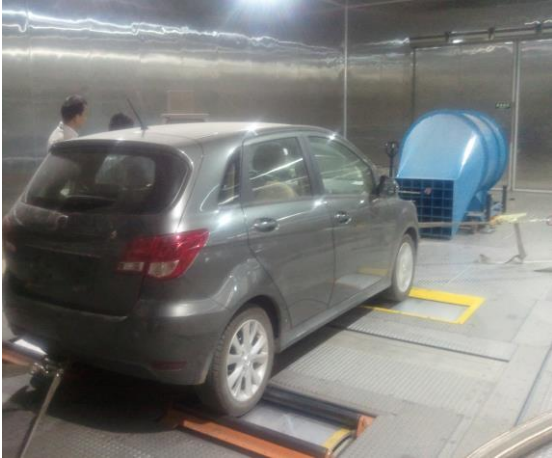
Figure 5: EV testing using a chassis dynamometer.
