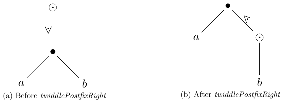
Figure A.4: twiddlePostfixRight tree transformation for representation of a \bullet b \odot where \odot is a postfix operator, \bullet is binary, and \odot \succ \bullet
