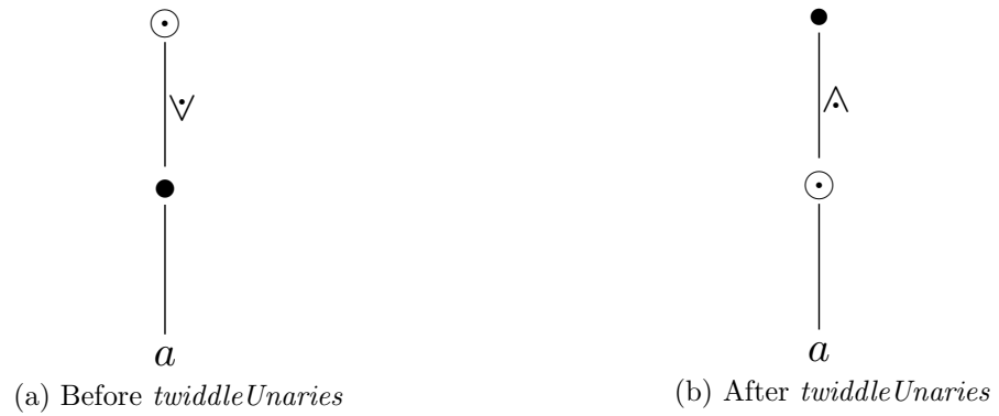
Figure A.7: twiddleUnaries tree transformation for representation of \odot a \bullet where \bullet is a postfix operator, \odot is prefix (or \bullet is prefix and \odot postfix), and \odot \succ \bullet
