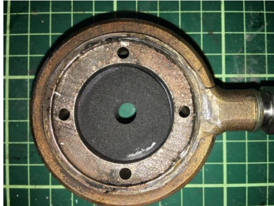
Figure 5b. Test 1 post firing nozzle and tangential injector
