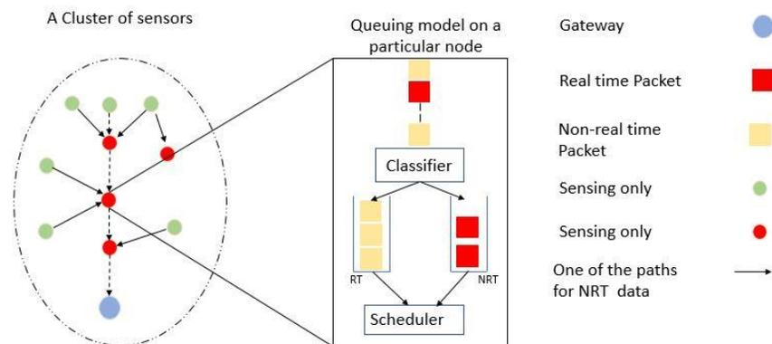
**Figure 1-3: Queuing model in cluster-based sensor network, Source: (Akkaya & Younis, 2005)**
