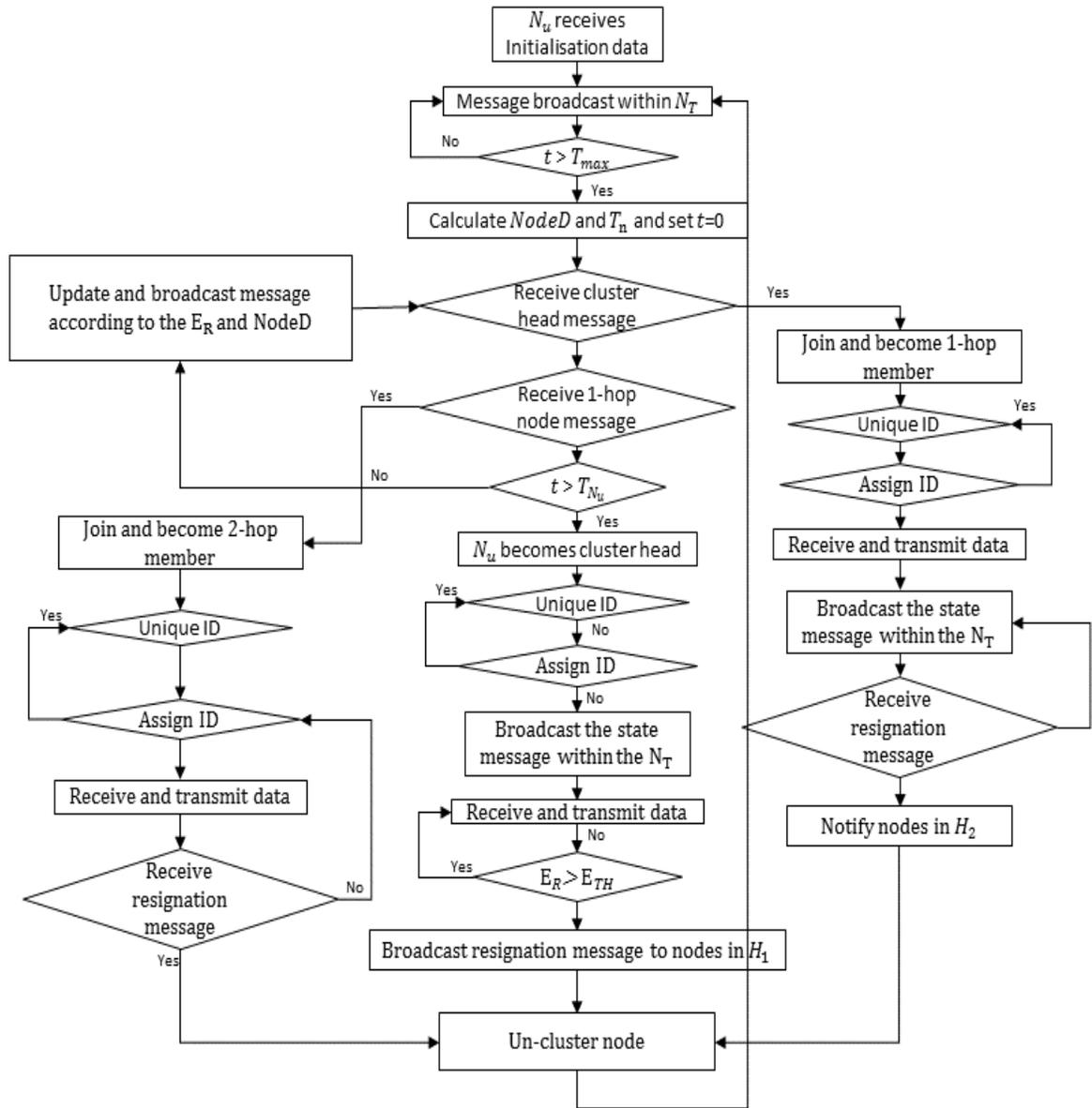
Figure 4-2 Flowchart of the EAAFC Algorithm
