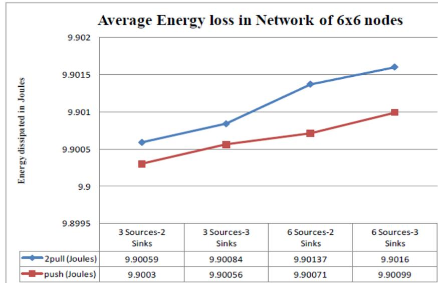
*Figure 3-5: The average energy dissipation in 6x6 nodes network*
