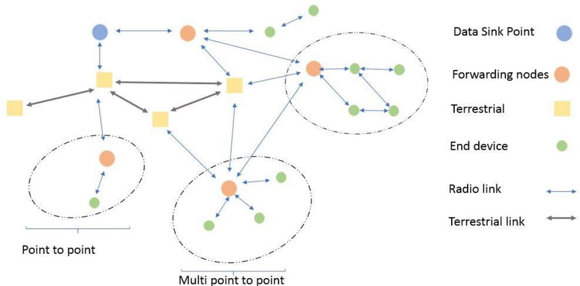
**Figure 1-2: C2WSNs: Point to point, typically single hop systems using static routing.**
