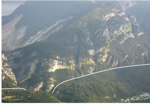
Figure 7. Left wall of the Piave Valley above Longarone in September 2011, showing the ‘chair’ structure (bedding indicated by yellow lines) that was mistakenly assumed to extend beneath at least the western half of the landslide. The white line marks the alignment of the Col delle Tosatte Fault. The downstream end of the Vaiont Gorge is at the lower left of the image and part of the landslide scar is visible in the upper left part. Photo: APD.
