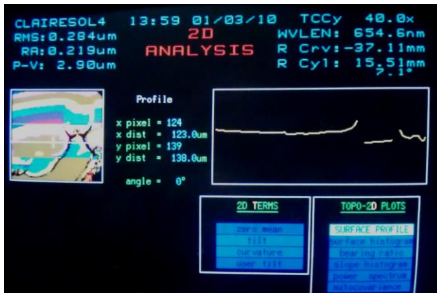
b. Interferometer screenshot image from a cross-section of a double layer of TiO 2 sol.
