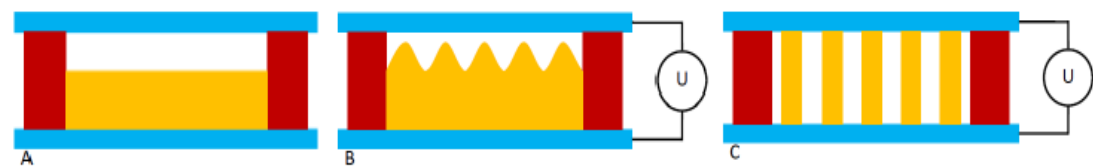
Figure 1. 15 Schematic of the EHD patterning process, blue - electrode, red - spacer, yellow - patternable fluid, A. no applied voltage B. initial instability C. fully evolved structures.
