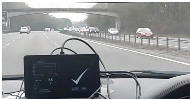
Figure 5.15: Driver feedback system mounted on test vehicle dashboard with recommended speed and gear along with feedback icon to maintain speed.
