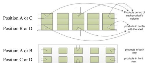
Fig. 4. Different positions of food products with thermocouples within the cabinet
