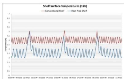
Fig. 7. Thermal profiles of the surface of conventional (red line) and heat pipe (blue line) shelves
