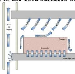
Fig. 2. Heat transfer mechanisms of the heat pipe shelf
