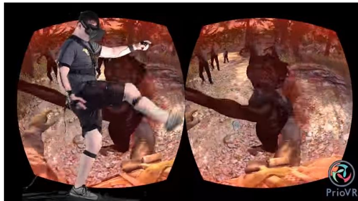
Figure 2-9 Overview of a body suit, currently under development designed for virtual reality or mo-cap at home. The body suit comprises of 17 inertial sensors and 2 hand controllers, to control the game character in conjunction with the Oculus rift to display the game to the player in 3D.
