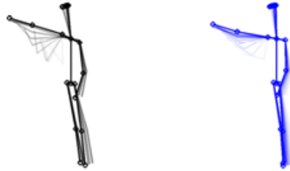
Figure 4-7 Template fragment matching: peak pose fragment (left), matched key pose fragment (right)
