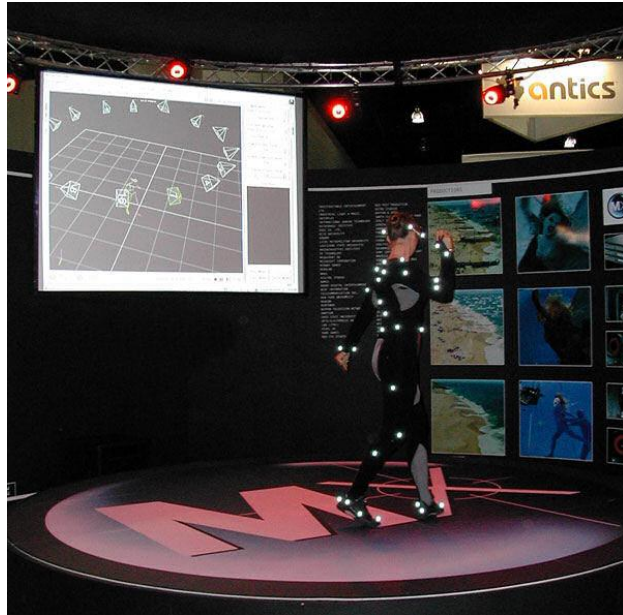
Figure 2-8 Overview of a commercial motion capture system. Multiple cameras are suspended from a rig in the ceiling, the subject has many markers on her body and the specialist software used for capturing and tracking the markers is shown.
