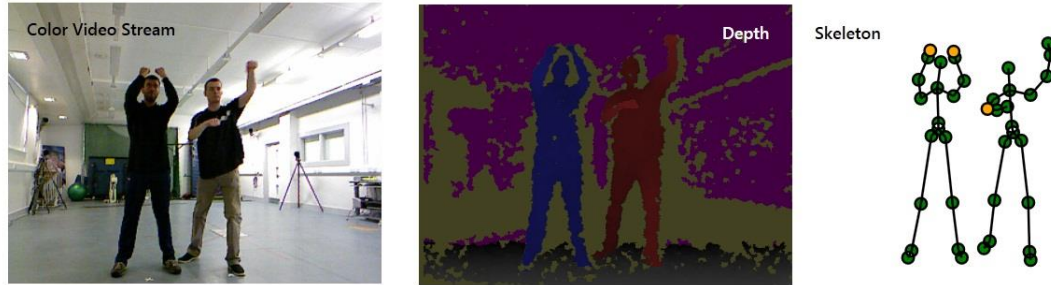
Figure 5-17 Synchronised colour, depth and skeleton data from a boxing game
