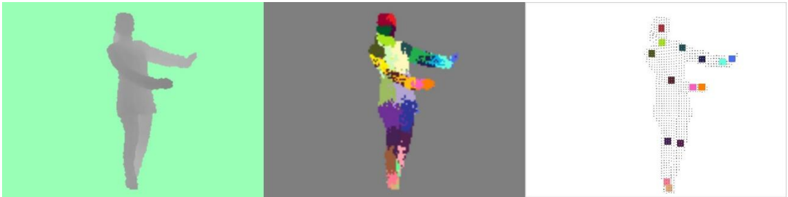
Figure 2-10 Overview of real-time pose recognition. From a single input depth image (left), a per-pixel body part distribution is inferred (middle), local modes are estimated to give proposals for the 3D locations of body joints (right) [6]
