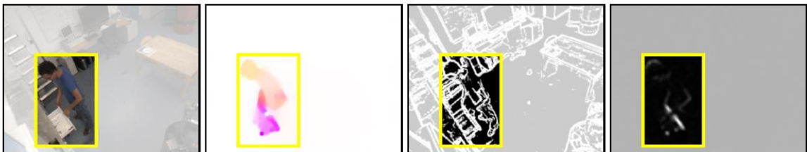
Figure 2-6 Appearance-based features, from left to right: colour, dense optical flow, spatial gradients and temporal gradients [7]
