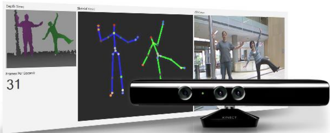
Figure 1-5 Microsoft Kinect (front) with depth (back left), skeleton (back middle) and RGB (back right) images [8]
