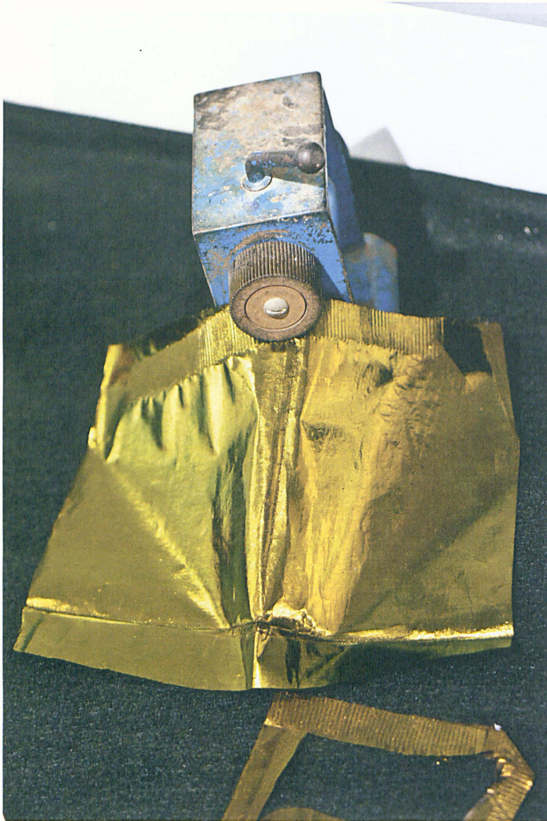
A Burqa Machine display in the open cabinet, this machine produced small-embossed straight lines that looked like the drapes on the forehead part of the burqa, 2014
