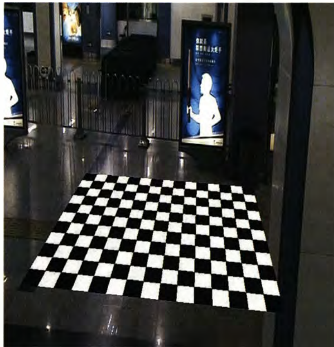
Figure 2.12: An artificially-made check board on top of tiles is used to perform camera calibration
