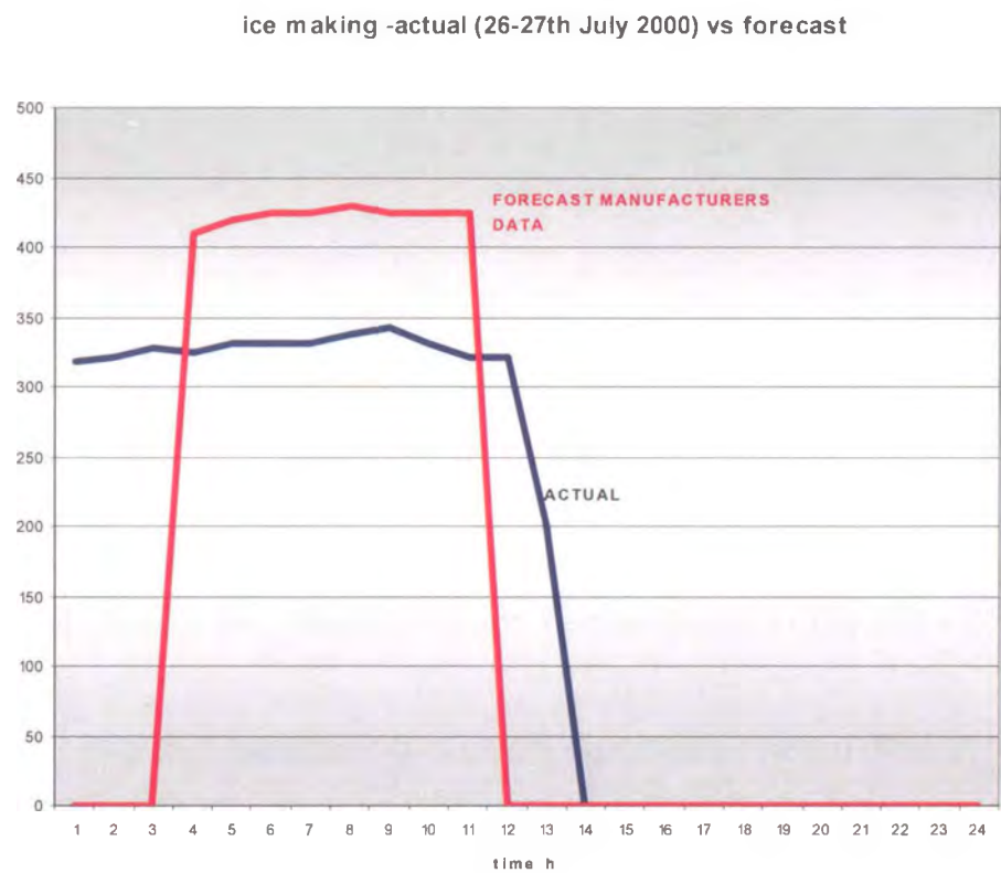
Fig.8.4 Chiller Actual Performance Against Manufacturer’s Data
