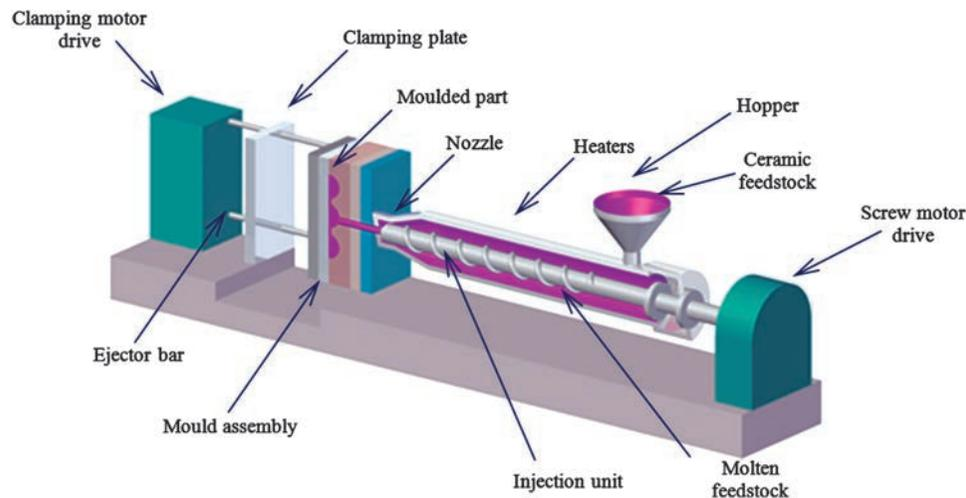
Figure 8. Schematic diagram of injection molding setup.
