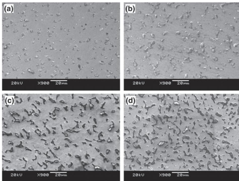
**Figure 26.** Composite stainless steel alumina micro parts using alumina content of (a) 2.5%; (b) 5%; (c) 7.5%; (d) 10%. Reprinted with permission from [40], M. F. Imbavy and K. Jiang, Fabrication of free standing 316-L stainless steel–Al<sub>2</sub>O<sub>3</sub> composite micro machine parts by soft molding. *Acta Materialia* 57, 4751 (2009). © 2009, Elsevier.
