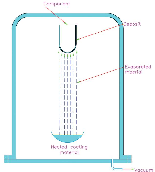
Figure 21. Schematic of physical vapor deposition.
