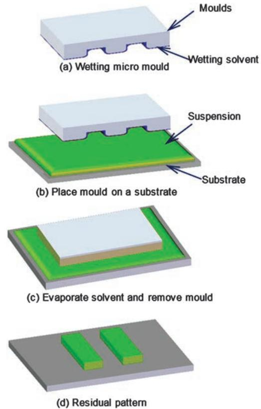
Figure 15. Schematic illustration of solvent-assisted micromolding process.
