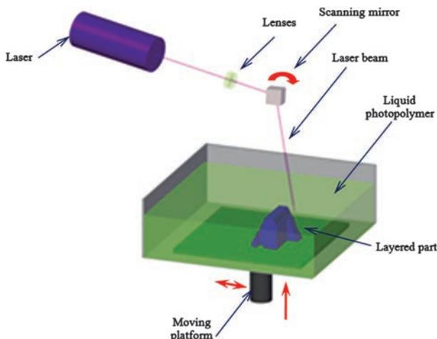
Figure 2. Schematic representation of stereolithography setup.
