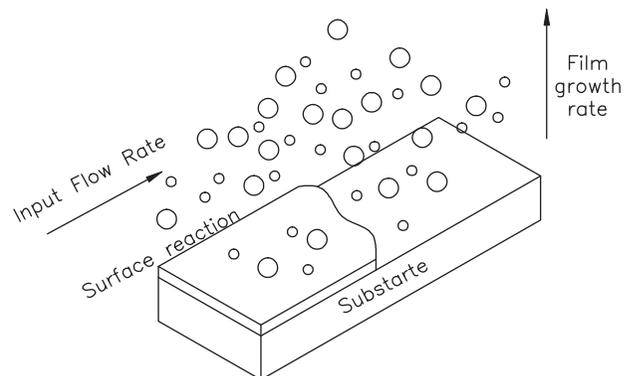
**Figure 20.** Chemical vapor deposition process.
