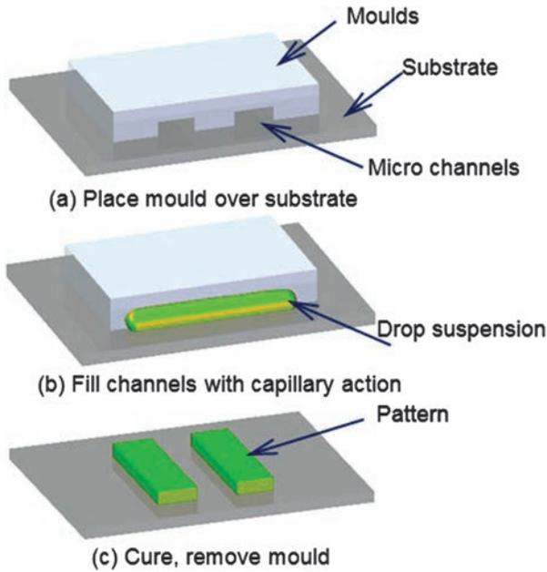
Figure 14. Schematic illustration of micromolding in capillaries process.
