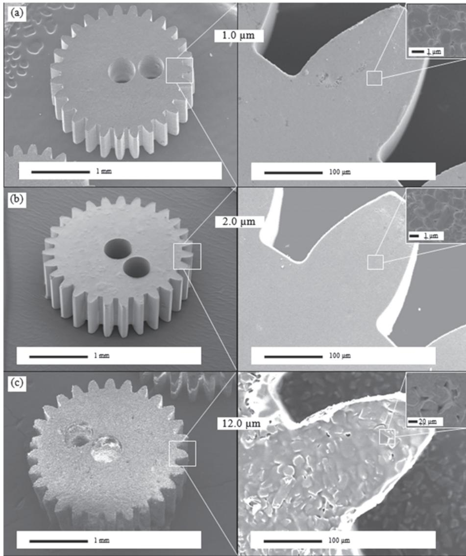
**Figure 23.** SEM images of ceramic micro parts using powder size of (a)  $1.0\ \mu\text{m}$ , (b)  $2.0\ \mu\text{m}$ , (c)  $12.0\ \mu\text{m}$ . Reprinted with permission from [212], H. Hassanin and K. Jiang, Effects of particle size on soft lithography process, the green and sintered micro alumina parts. *International Journal of Applied Ceramic Technology* 10, 1014 (2013). © 2013, John Wiley and Sons.
