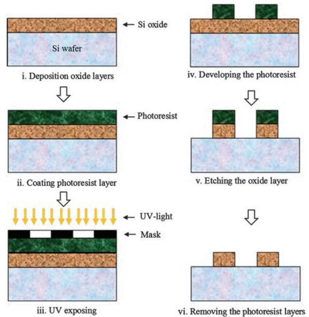
**Figure 17.** Schematic diagram showing the etching micromachining process.
