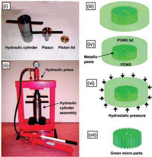
**Figure 16.** Schematic diagram of the cold isostatic pressing technique. Reprinted with permission from [176], M. Imbaby, et al., Fabrication of 316-L stainless steel microcomponents using encapsulating soft mold and isopressing technique. *Microelectronic Engineering* 87, 1623 (2010). © 2010, Elsevier.
