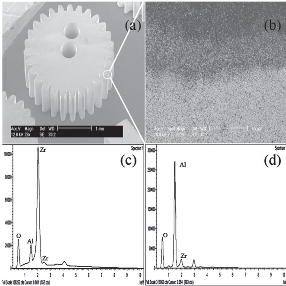
**Figure 27.** SEM of a FGM micro gear, (b) BSE of the interface, (c) EDS of the dark area, (D) EDS of bright area. Reprinted with permission from [46] H. Hassanin and K. Jiang, Functionally graded microceramic components. *Microelectronic Engineering* 87, 1610 (2010). © 2010, Elsevier.
