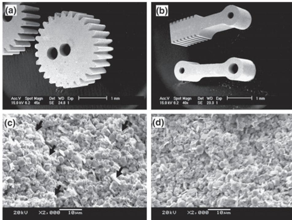
**Figure 25.** Composite micro parts: (a) micro gears; (b) micro pistons. Fractured surface of 10% alumina composite: (c) dispersed powders together; (d) powders dispersed separately. Reprinted with permission from [40] M. F. Imbady and K. Jiang, Fabrication of free standing 316-L stainless steel– $\text{Al}_2\text{O}_3$  composite micro machine parts by soft molding. *Acta Materialia* 57, 4751 (2009). © 2009, Elsevier.
