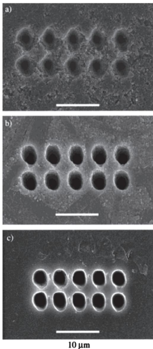
**Figure 22.** Ceramic cavities fabricated with an average diameter of (a)  $0.5\ \mu\text{m}$ , (b)  $0.2\ \mu\text{m}$ , (c)  $45\ \text{nm}$ . Reprinted with permission from [211], U. P. Schonholzer, et al., Microfabrication of ceramics by filling of photoresist molds. *Advanced Materials*, (2000). © 2000, John Wiley and Sons.
