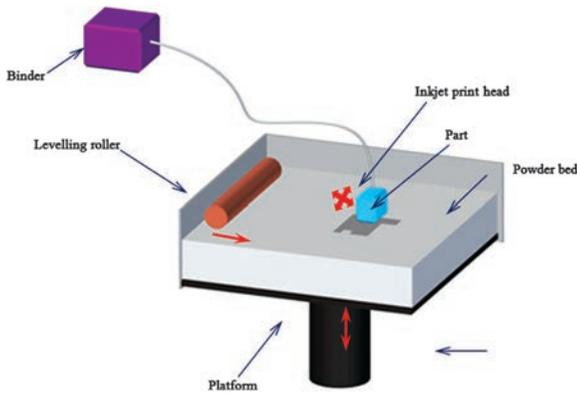
Figure 6. Schematic diagram of powder bed jet system.
