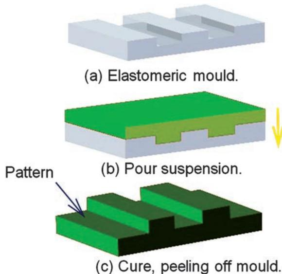
Figure 12. Schematic illustration of replica molding process.
