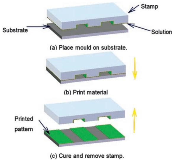
Figure 11. Schematic illustration of the general process of microcontact printing.
