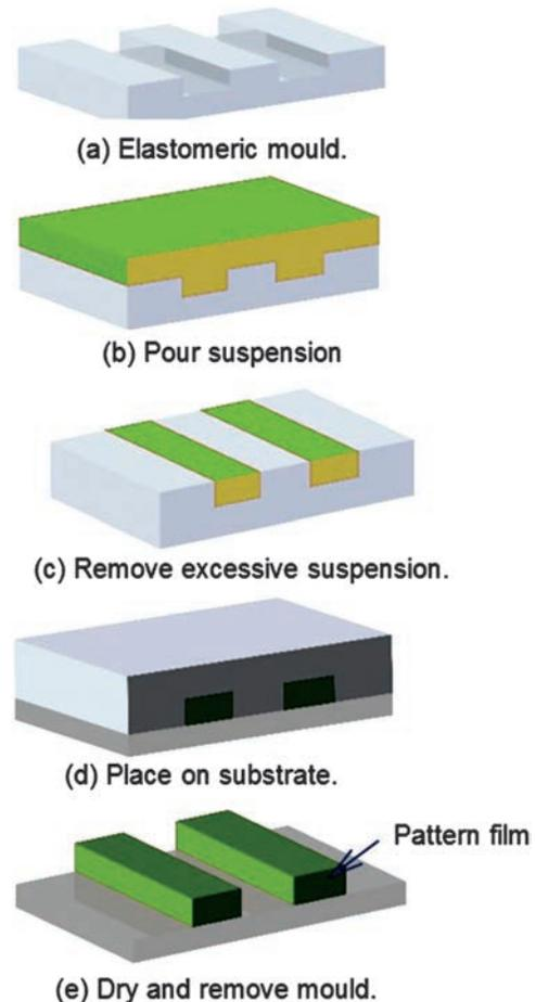
Figure 13. Schematic illustration of microtransfer molding process.
