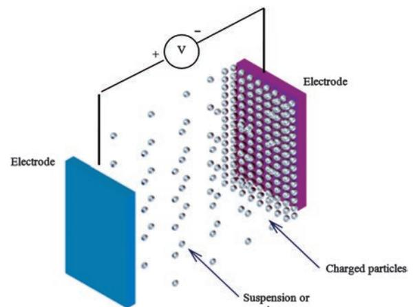
Figure 9. Schematic diagram of electrophoretic deposition and electroforming principal.
