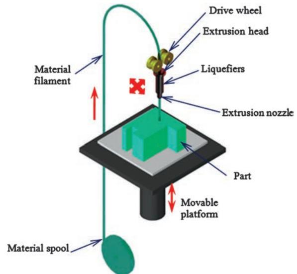
Figure 3. Schematic diagram of the fused deposition process.
