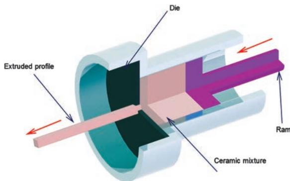
Figure 10. Schematic diagram of coextrusion process.
