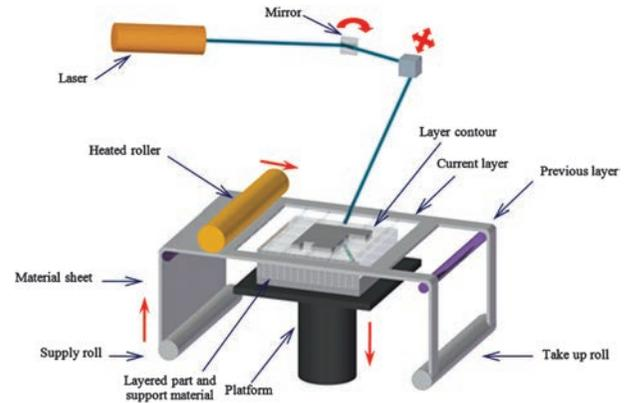
Figure 5. Schematic diagram of laminated object manufacturing process.
