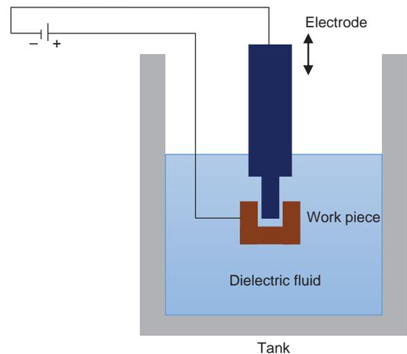
**Figure 18.** Schematic diagram showing microelectrical discharge machining.
