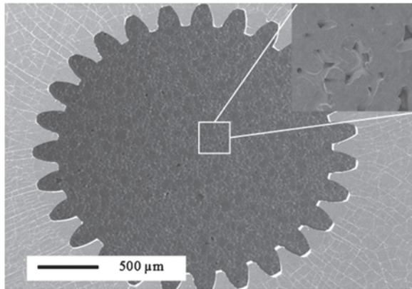
**Figure 24.** SEM image of PDMS through mold placed on a porous substrate. Reprinted with permission from [226], H. Hassanin and K. Jiang, Fabrication and characterization of stabilized zirconia micro parts via slip casting and soft molding. *Scripta Materialia* 69, 433 (2013). © 2013, Elsevier.
