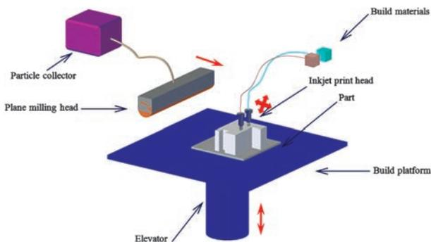
Figure 7. Schematic diagram of ink jet printing process.
