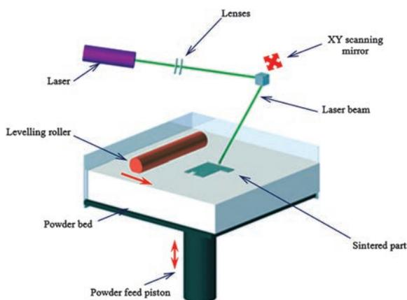
Figure 4. Schematic diagram of selective laser melting process.
