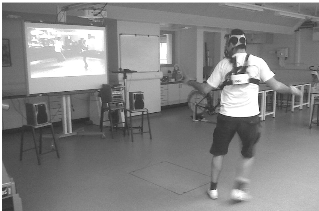
Figure 3.1. A participant performing the laboratory-based dance trial to the choreography video in Study 1 using the K4b 2 portable indirect calorimeter (photographic permission given by the participant for use in this thesis).
