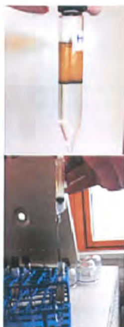
Figure 3.9: Analytes extraction using a mixture of solvents after centrifugation.
