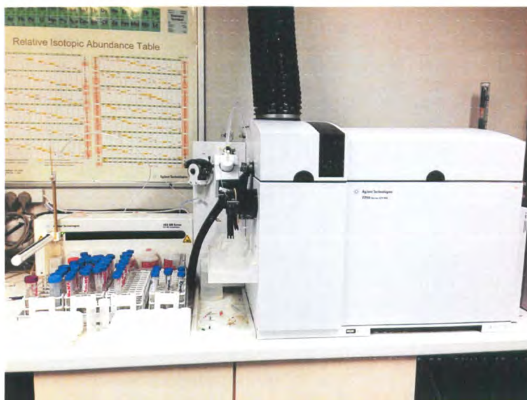
Figure 0.15: AGILENT Technology (Agilent 7700) inductively coupled plasma mass spectrometry (ICP-MS)
