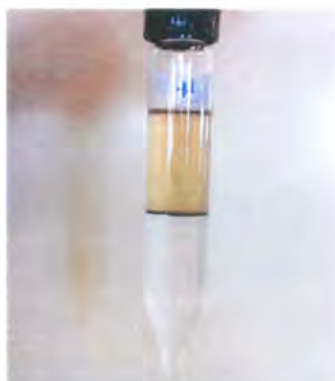
Figure 0.3: Photo image of the extraction procedure using (3:1:1) chloroform, ethanol and ethyl acetate.
