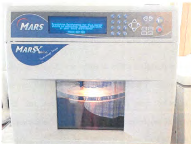
Figure 0.12: MARS X microwave used in the rubber digestion and the digested sample
