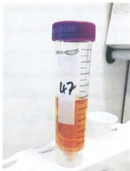
Figure 0.13: Digested tyre rubber sample.
