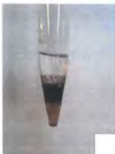
Figure 0.6: LLE of a hair sample using pentane.
