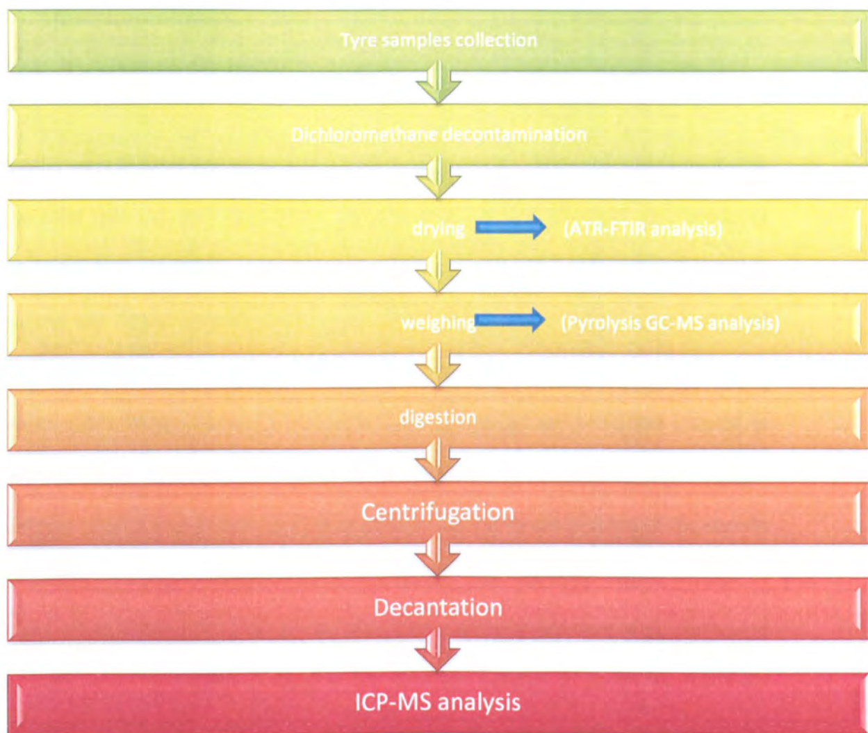
Figure 7.2: Rubber samples analysis process.
