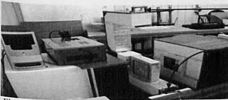
Figure 3-13 Hot box components separated and the sample carrier open showing a sample in place.
