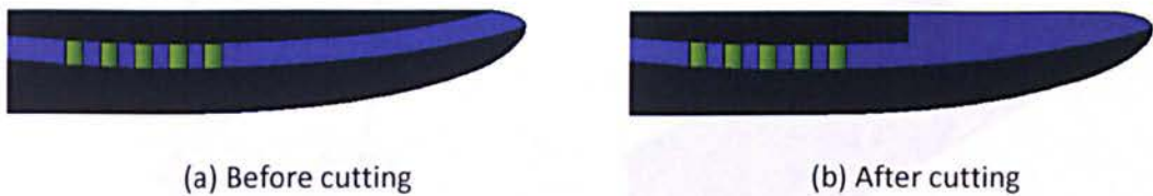
Figure 2–2: Cutting process of trailing-edge.
