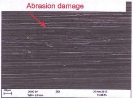
Figure 5.23. (A,C) SEM micrographs of wear scars on Nitinol pin and (B,D) titanium disk in Nitinol – Ti6Al4V friction combination in case of ion implantation performed on both components (Test 6): A) and B) after 2,000 cycles; C and D after wear test termination at 0.85 million cycles (C and D)
