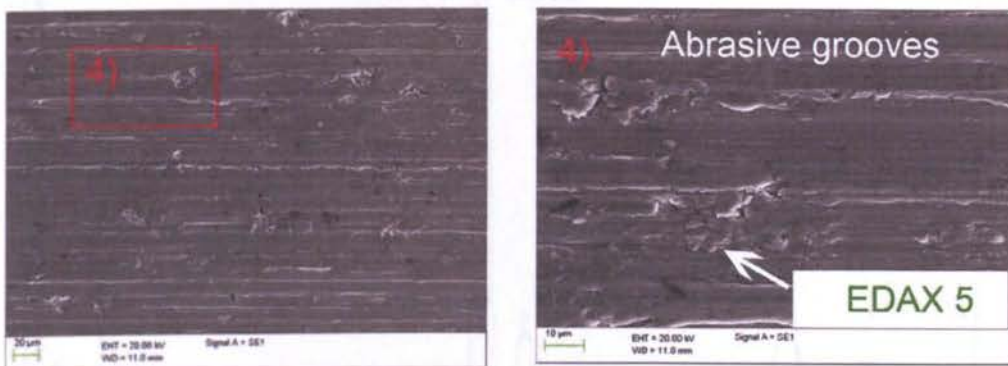
Fig. 4.8. SEM of wear scars on Nitinol pin (A and B) and titanium disk (C and D) in Nitinol - Ti6Al4V friction combination components after 0.1 million cycles of testing
