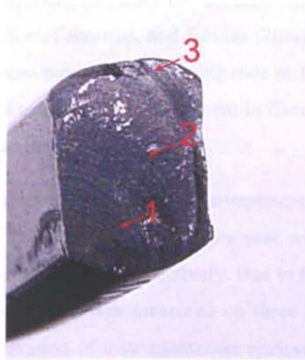
Figure 2.17 Fracture surface of the rod in patient P. 4R after 1.5 years of implantation reveals features of fatigue failure: crack initiation site (1), propagation zone (2) and rupture zone (3).
