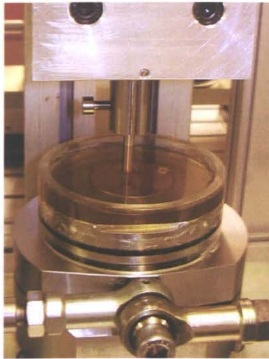
Figure 4.2. Photo of pin-on-disk wear test for the in-vitro evaluation of wear resistance of Ti6Al4V – Ti6Al4V, Nitinol- Ti6Al4V and CoCr – Ti6Al4V friction combinations
