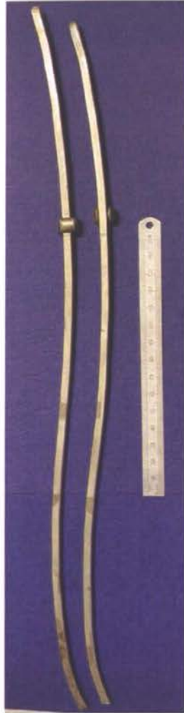
Figure 2.4. Photos of retrieved rods of LSZ-4D sliding device for EOS: (A) overall view of rods; (B) cervical region of rods; (C) thoracic region of rods; (D) lumbar region of rods. Implant retrieved from patient P.1R (5.8 years of implantation).
