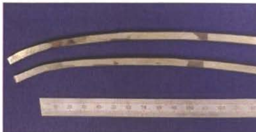
Figure 2.4. Photos of retrieved rods of LSZ-4D sliding device for EOS: (A) overall view of rods; (B) cervical region of rods; (C) thoracic region of rods; (D) lumbar region of rods. Implant retrieved from patient P.1R (5.8 years of implantation).
