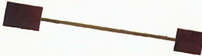
Figure 3.13: Calibration tool for creating corresponding planes – the “paddle”.
