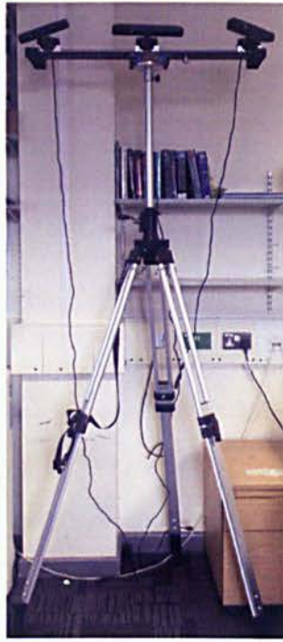
Figure 3.7: Tripod and camera mounting set up.
