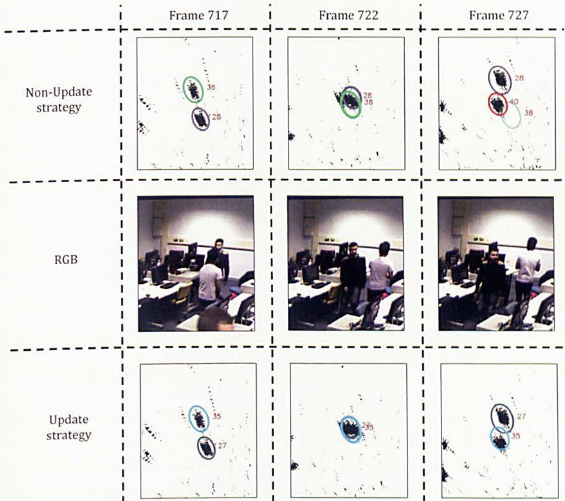
Figure 6.8: Three key frames of an interaction period between two targets. Top row: Non-update strategy combined with spatial models and INN. This approach fails as the motion of one of the targets slightly changes during the interaction. Middle row: Colour images of the key frames of the interaction. Bottom row: Update strategy combined with chromograms and GNN. In this case the association is resolved successfully.
