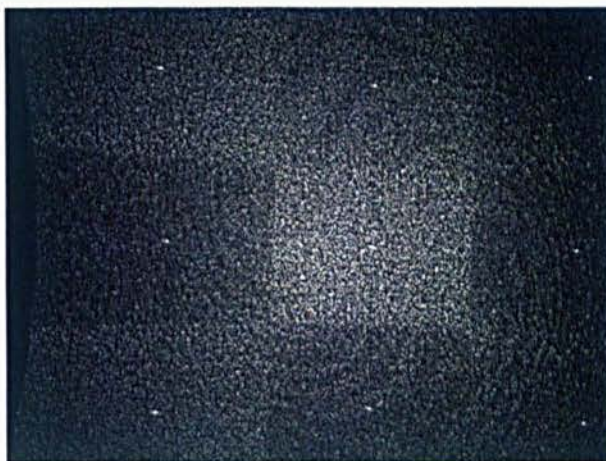
Figure 3.1: Infra-red image from Kinect sensor.
