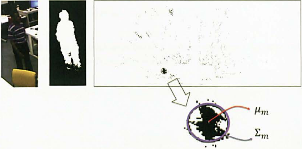
Figure 5.3: Spatial appearance model of a measurement. The RGB representation of the target is displayed in the most left image, followed by its segmentation in the IPS and the projection of all its constituent points into the MoA. Besides, the MoA projection is enlarged to present the spatial model of the measurement (mean and covariance of the projections distribution).
