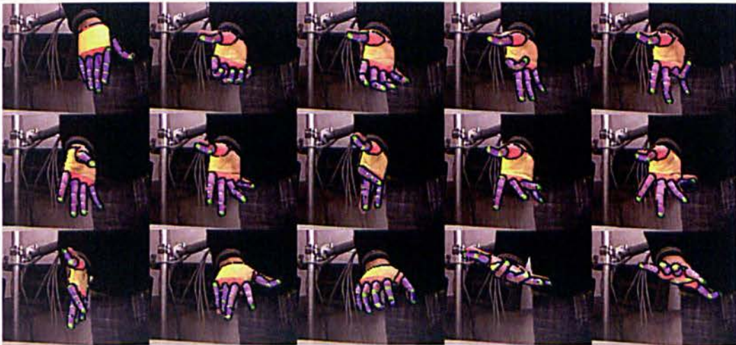
Figure 2.11: Hand articulation real time tracking and reconstruction using Kinect (Oikonomidis et al., 2011).
