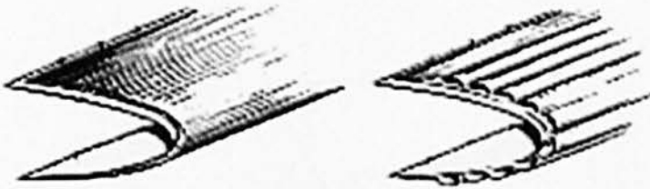
Figure 2.2.1: Construction and operation of pneumatic inflatable boots [21]
