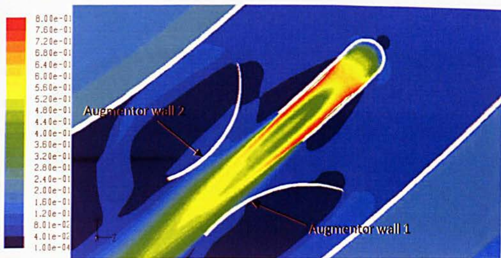
Figure 6.1.5: Contour of Mach number in augmentor vicinity
