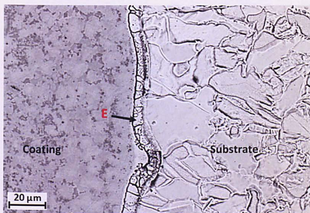
Fig. 7.5. Microstructure across the interface in the TiC system
