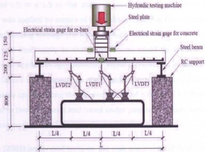
Figure 2-23 Arrangements for testing a Slab Specimen (Nguyen et al 2010)
