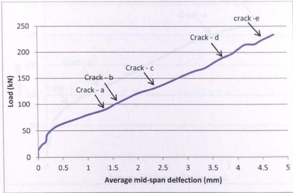
Figure 5-19 Average mid span deflection of 70PC/30PFA
