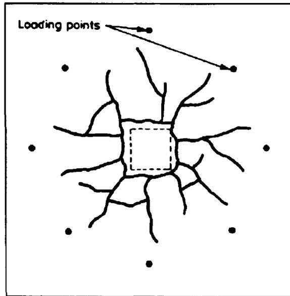
**Figure 2-19 Typical Crack pattern at failure Chana & Desai (1992)**
