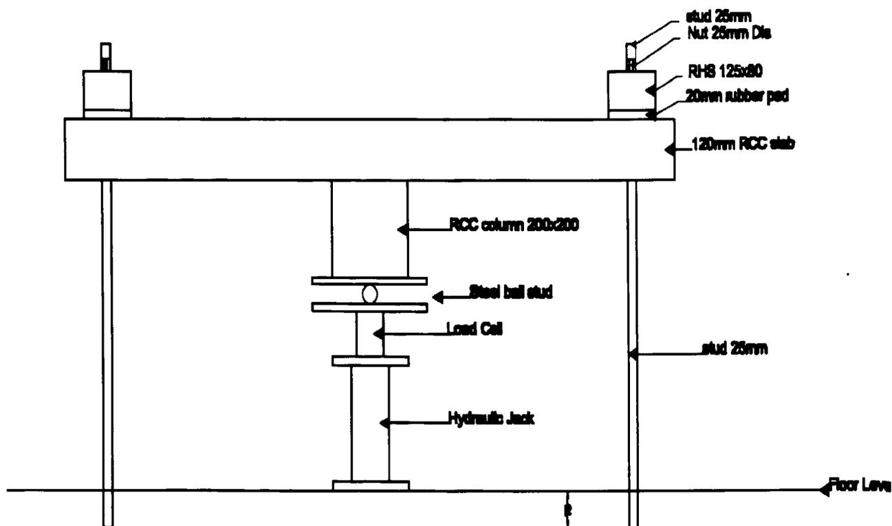
Figure 3-23 Testing rig arrangement for punching shear strength
