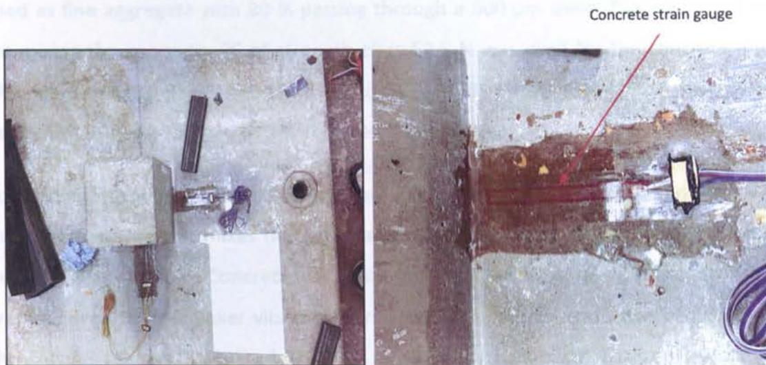
**Figure 3-17 Concrete strain gauges**
