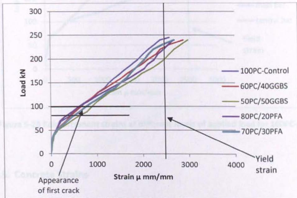
**Figure 5-22 Reinforcement strains at different levels of applied load**
