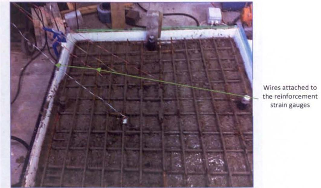
Figure 3-20 casting of slab specimen
