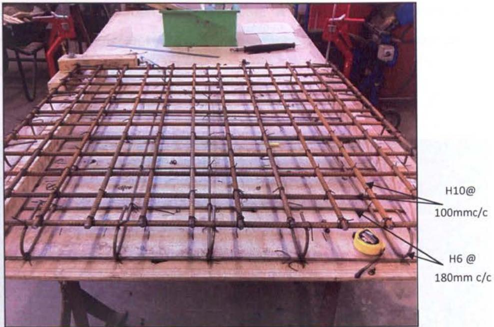
Figure 3-15 Reinforcement cage for slab specimen
