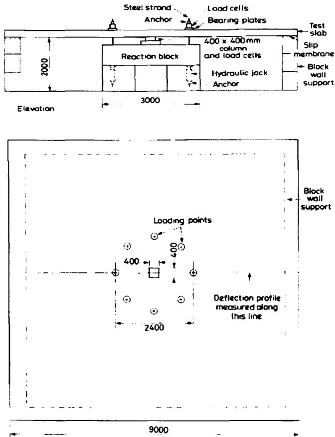
Figure 2-17 Schematic of Test arrangements (Chana & Desai, 1992)
