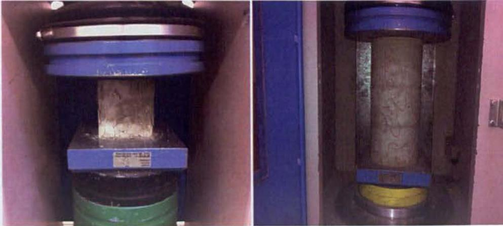
**Figure 3-9 Compressive strength Test (Cube and cylinder)**
