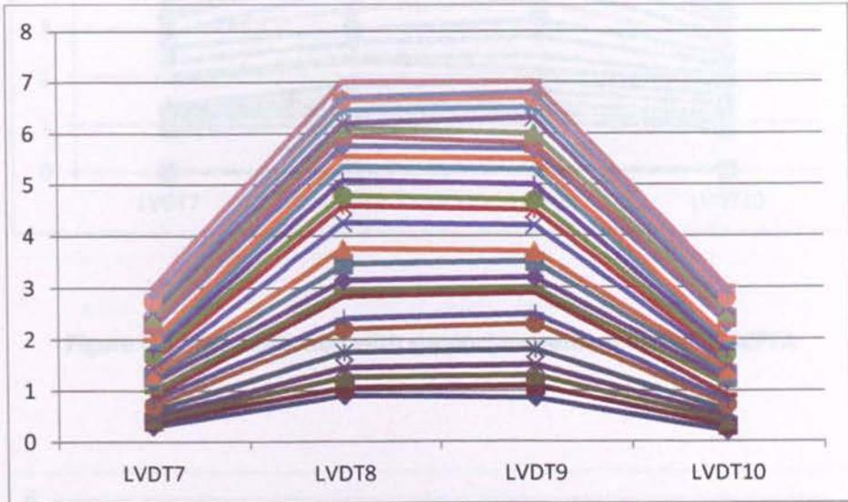
Figure C-1 Slab deflection with support movement for 100PC-Control
