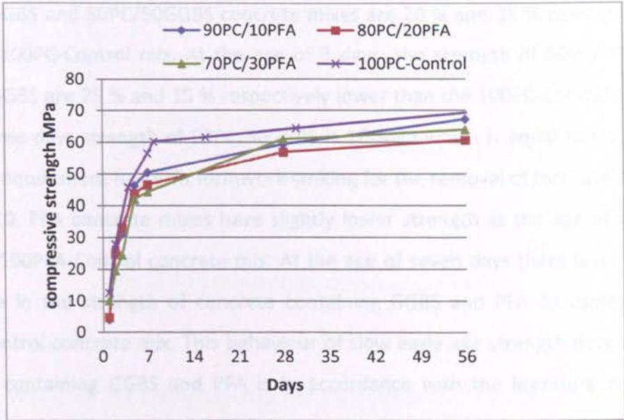
**Figure 4-11** Compressive strength development of PFA concrete mixes for C2
