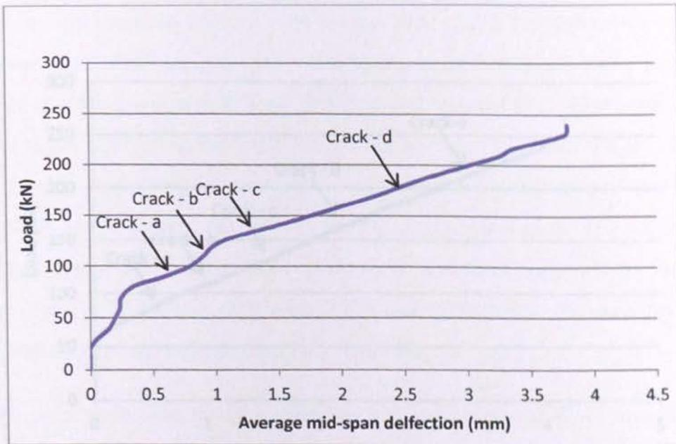
Figure 5-18 Average mid span deflection of 80PC/20PFA
