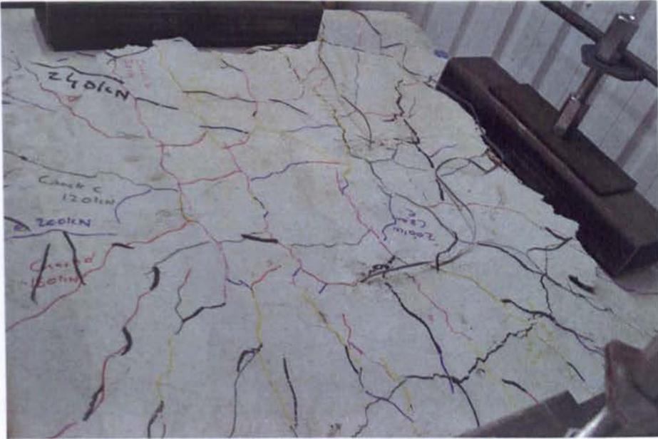
**Figure 5-7 60PC/40GGBS slab specimen after failure**
