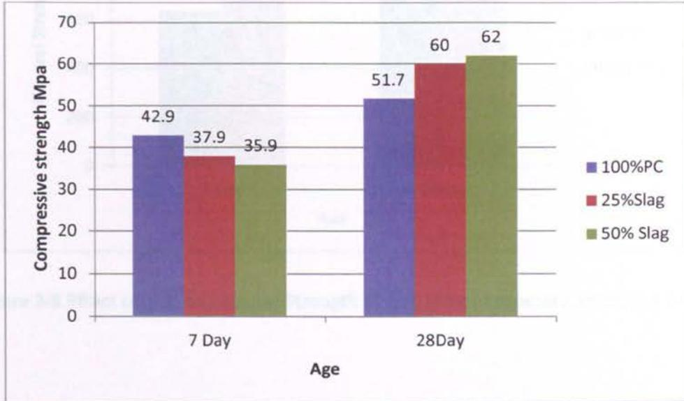
Figure 2-4 Effect of Slag on Compressive strength of slag cement concrete after (SCA 2003)
