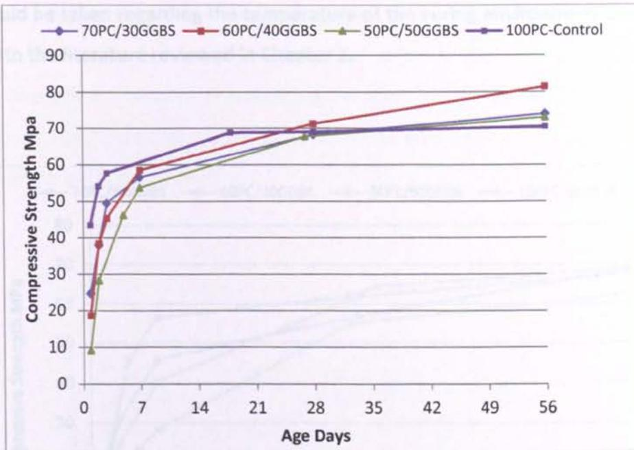
**Figure 4-1** Compressive strength development of GGBS concrete cured at C1 environment
