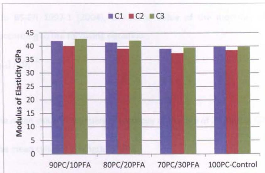
**Figure 4-16** Modulus of elasticity of PFA concrete at the age of 28 days
