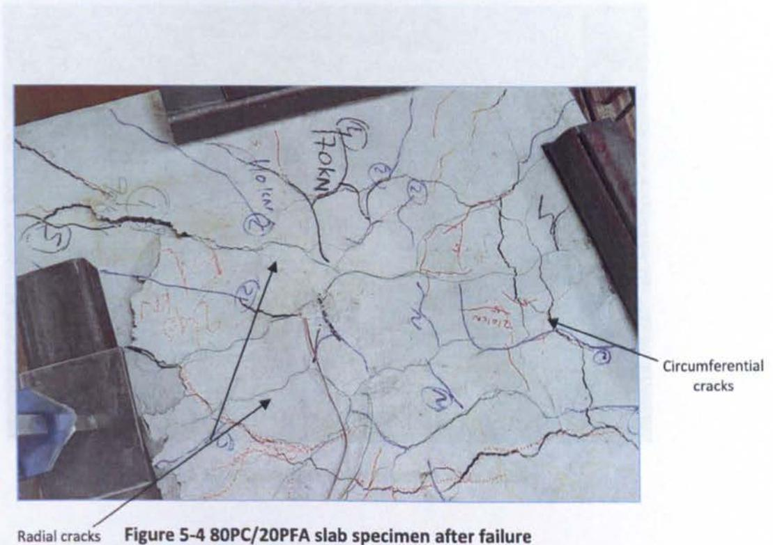
Radial cracks **Figure 5-4 80PC/20PFA slab specimen after failure**
