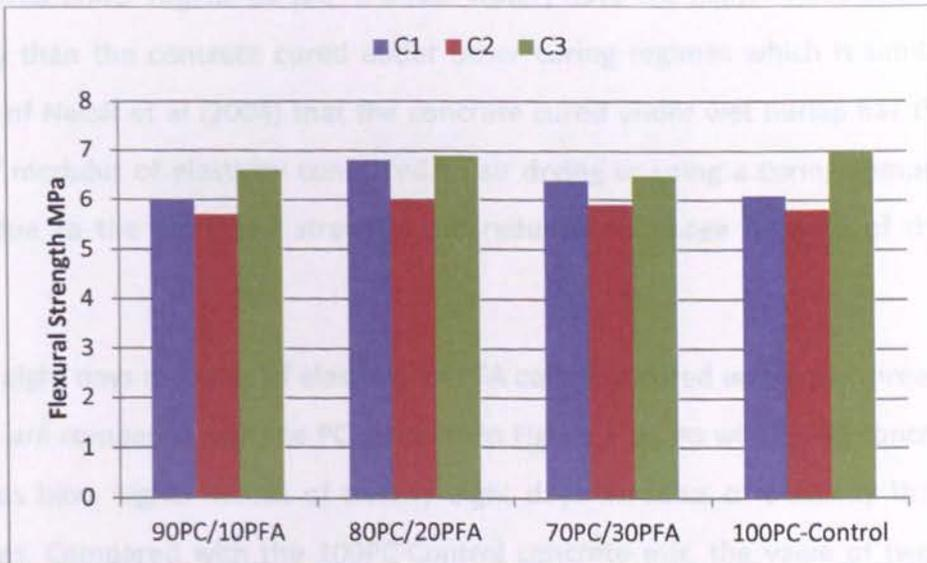
Figure 4-14 Flexural strength of PFA concrete at the age of 28 days
