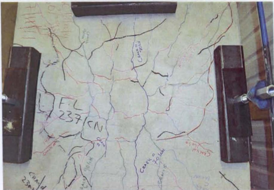
**Figure 5-8 50PC/50GGBS slab specimen after failure**
