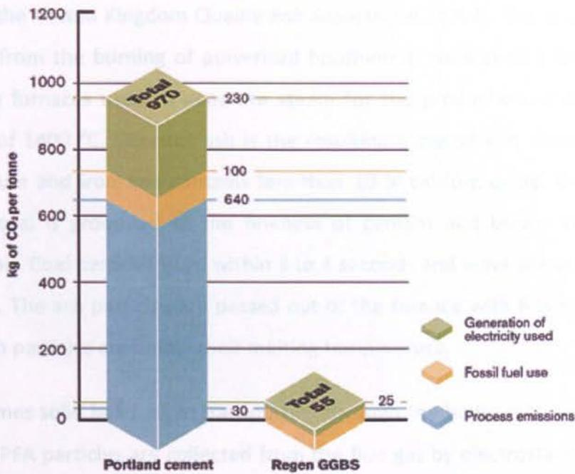
Figure 2-9 Typical CO<sub>2</sub> emissions for Portland cement and GGBS (Hanson 2010)
