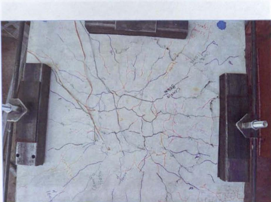
**Figure 5-6 100PC-Control slab specimen after failure**
