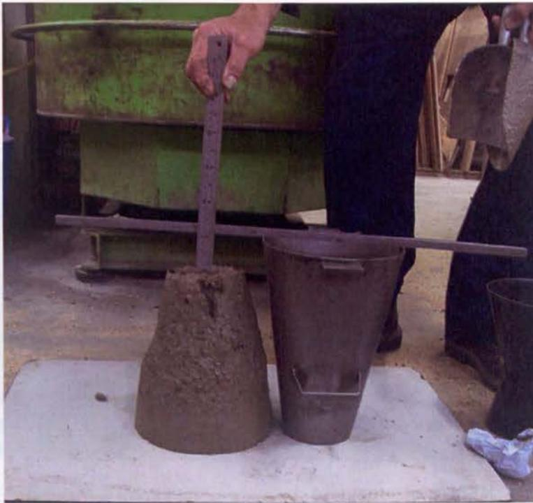
Figure 3-8 Slump test
