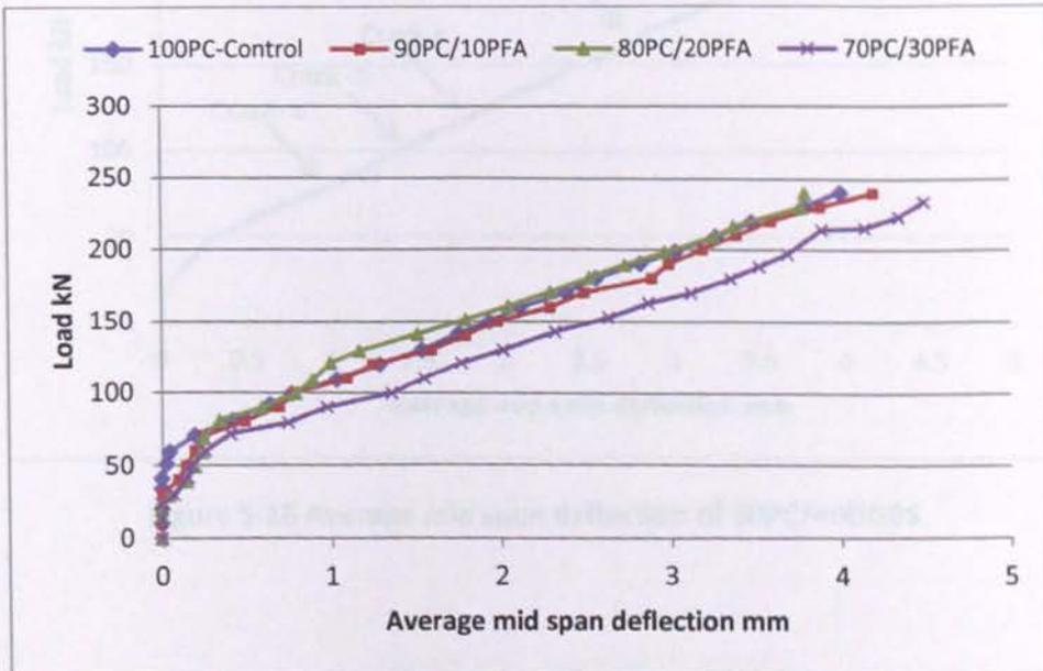
Figure 5-15 Average mid span deflection of PFA mixes
