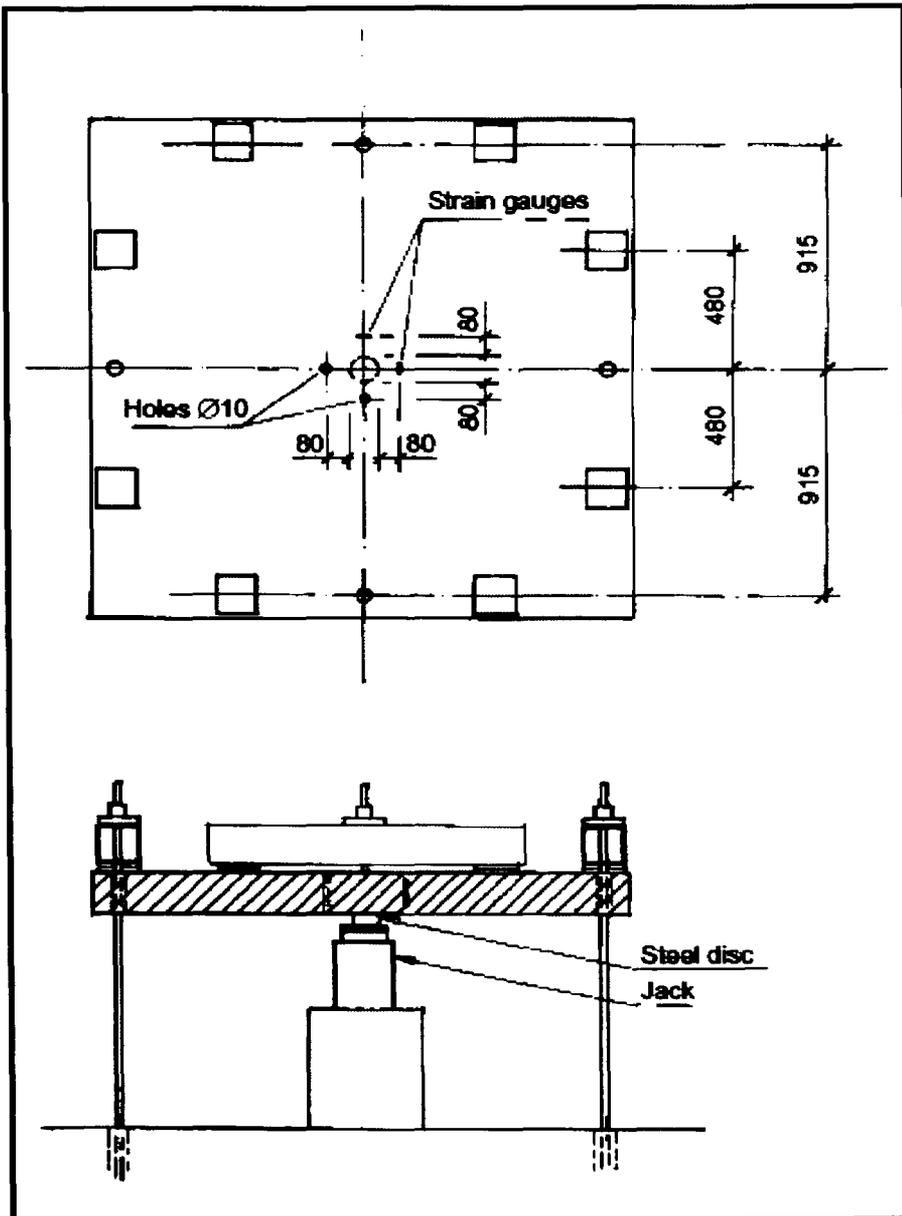
Figure 2-26 Punching shear test Arrangement (Regan 2003)
