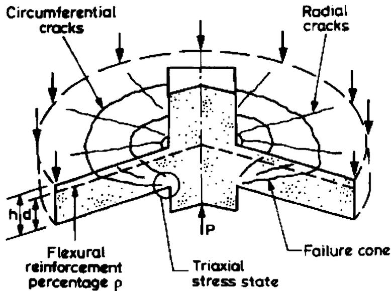
Figure 2-16 Crack Pattern Chana (1991)
