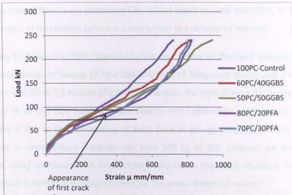
**Figure 5-24 Concrete Strains at different levels of applied load**
