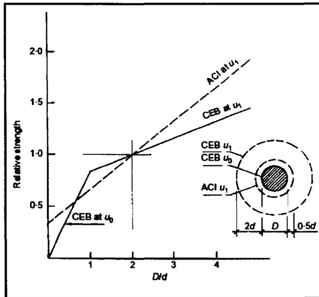
Figure 2-21 Effects of column size on punching shear strength (Regan 2003)
