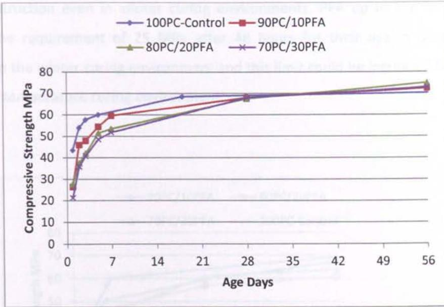
**Figure 4-10** Compressive strength development of PFA concrete for C1
