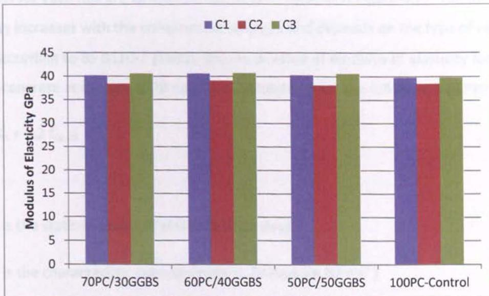
**Figure 4-15** Modulus of elasticity of GGBS concrete at the age of 28 days
