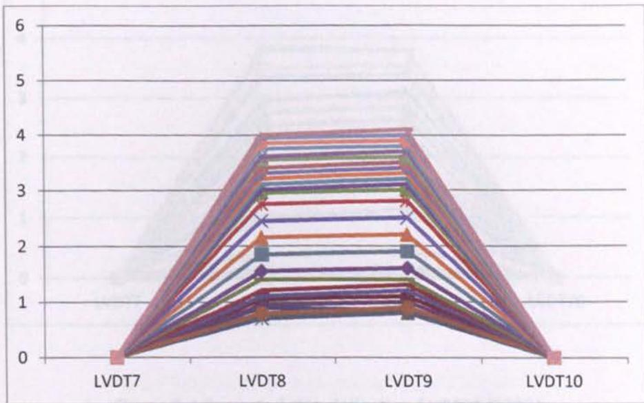
Figure C-2 Corrected slab deflection for 100PC-Control
