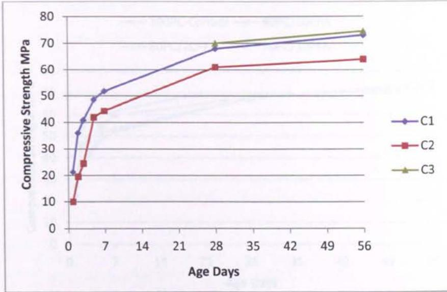
Figure 4-9 Compressive strength development of 70PC/30PFA concrete mix
