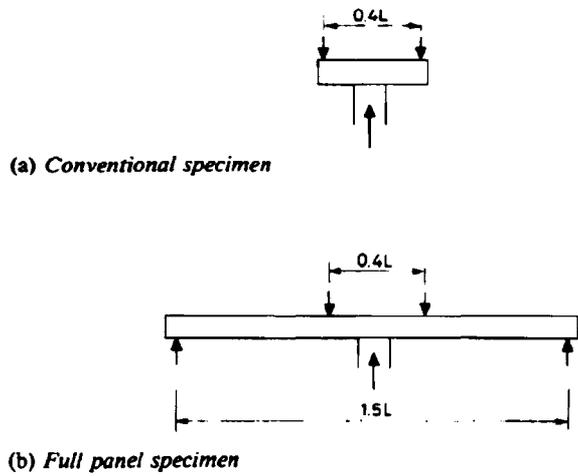
Figure 2-18 Comparison of slab test specimens, Chana & Desai (1992)
