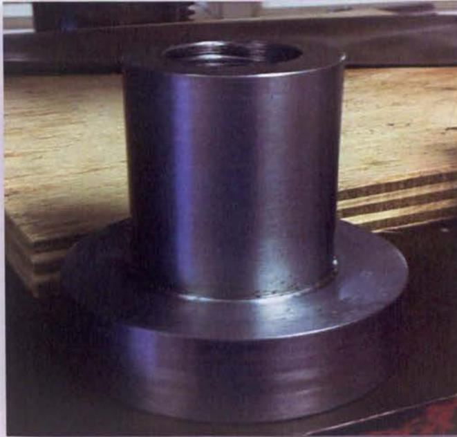
Figure 3-18 Inserts for making hole in the slab
