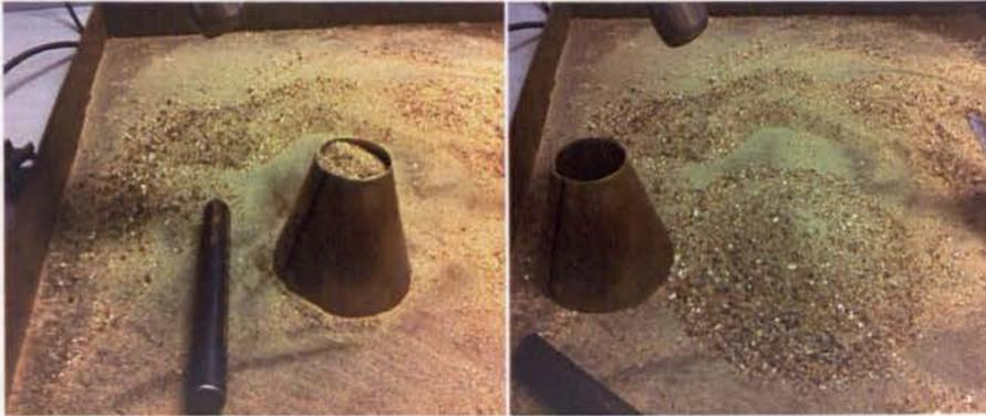
Figure 3-3 Aggregate drying in water absorption test
