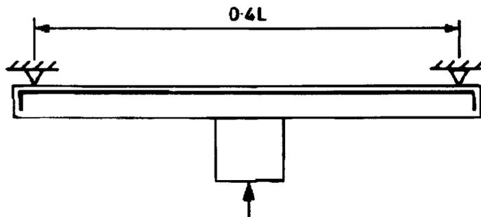
**Figure 2-15 Conventional Punching shear specimen Chana (1991)**
