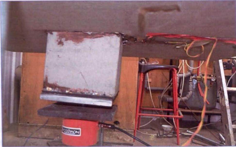
**Figure 5-11 50PC/50GGBS Punched column in the slab after failure**
