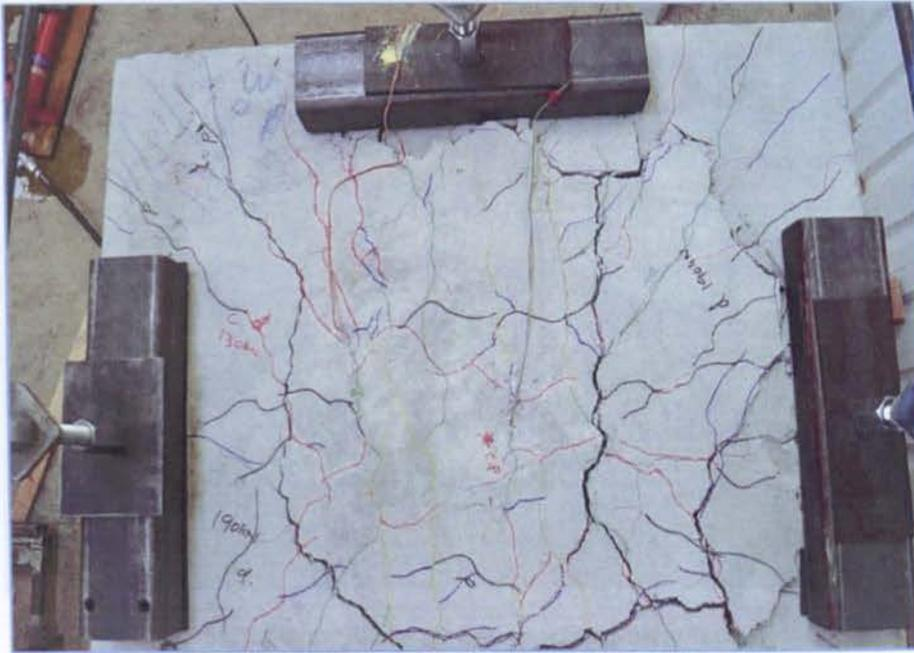
**Figure 5-5 70PC/30PFA slab specimen after failure**
