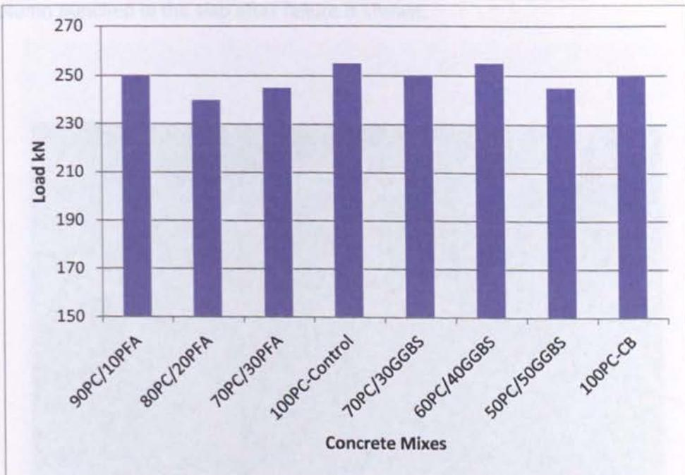
**Figure 5-3 Experimental Punching Shear failure Loads**
