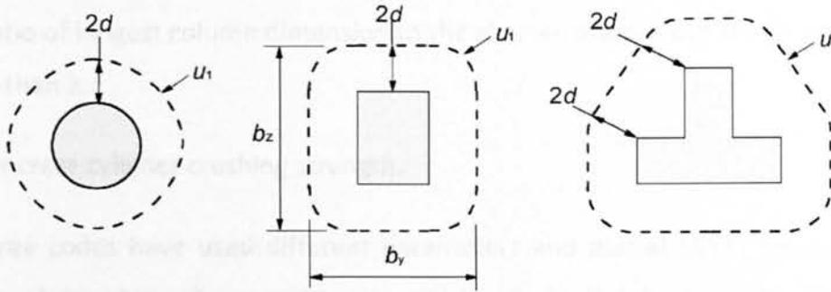
Figure 2-27 Typical basic control perimeters around loaded areas
