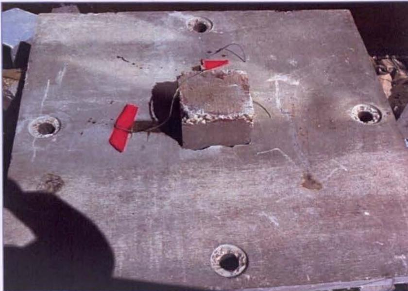
**Figure 3-22 Bottom surface of slab after failure**
