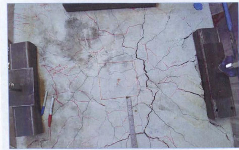
Figure 5-9 100PC-CB slab specimen after failure
