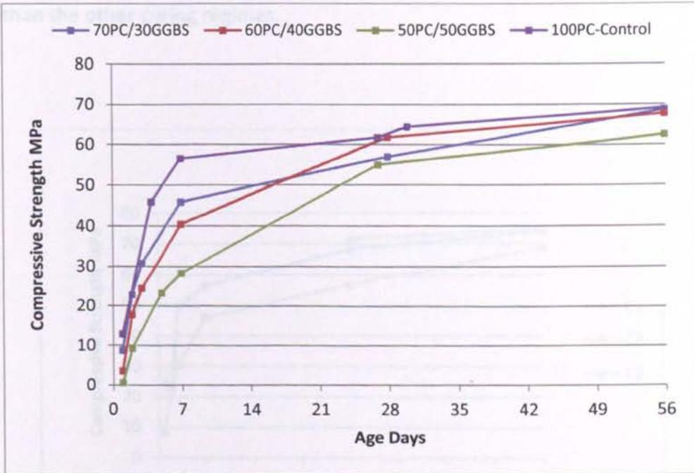
**Figure 4-2** Compressive strength development of GGBS concrete cured at C2 environment
