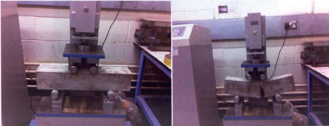
Figure 3-10 Flexural strength test
