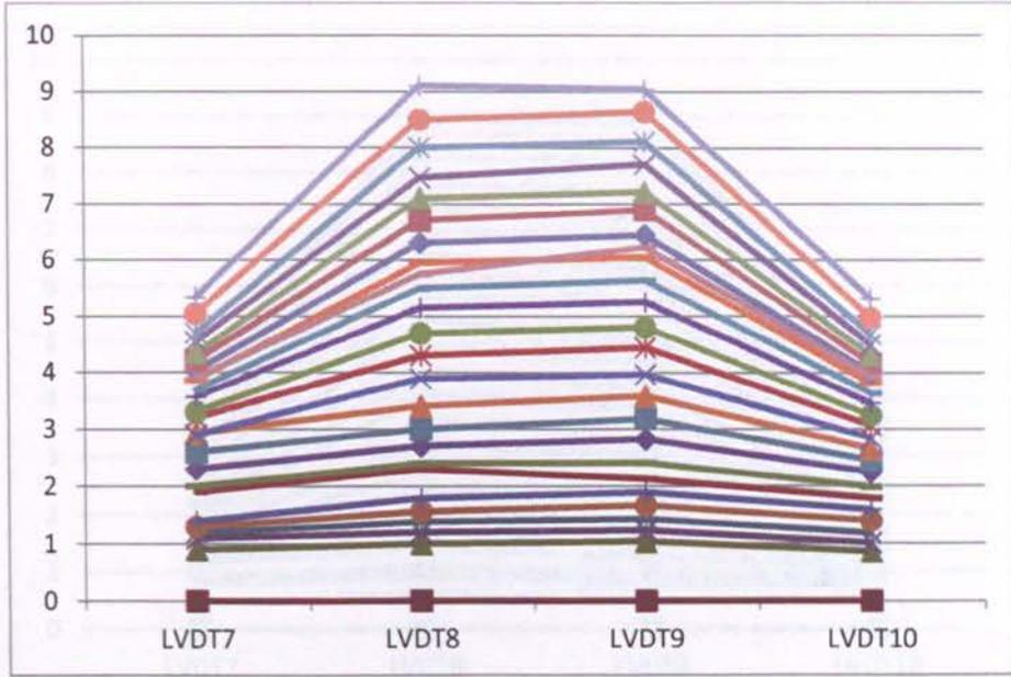
Figure C-3 Slab deflection with support movement for 80PC/20PFA
