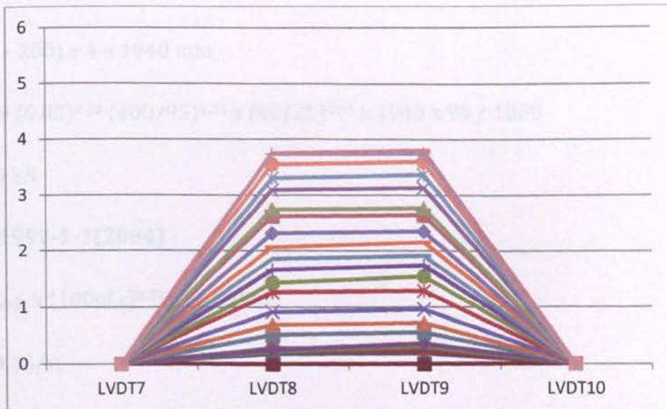
Figure C-12 Corrected slab deflection for 100PC-CB
