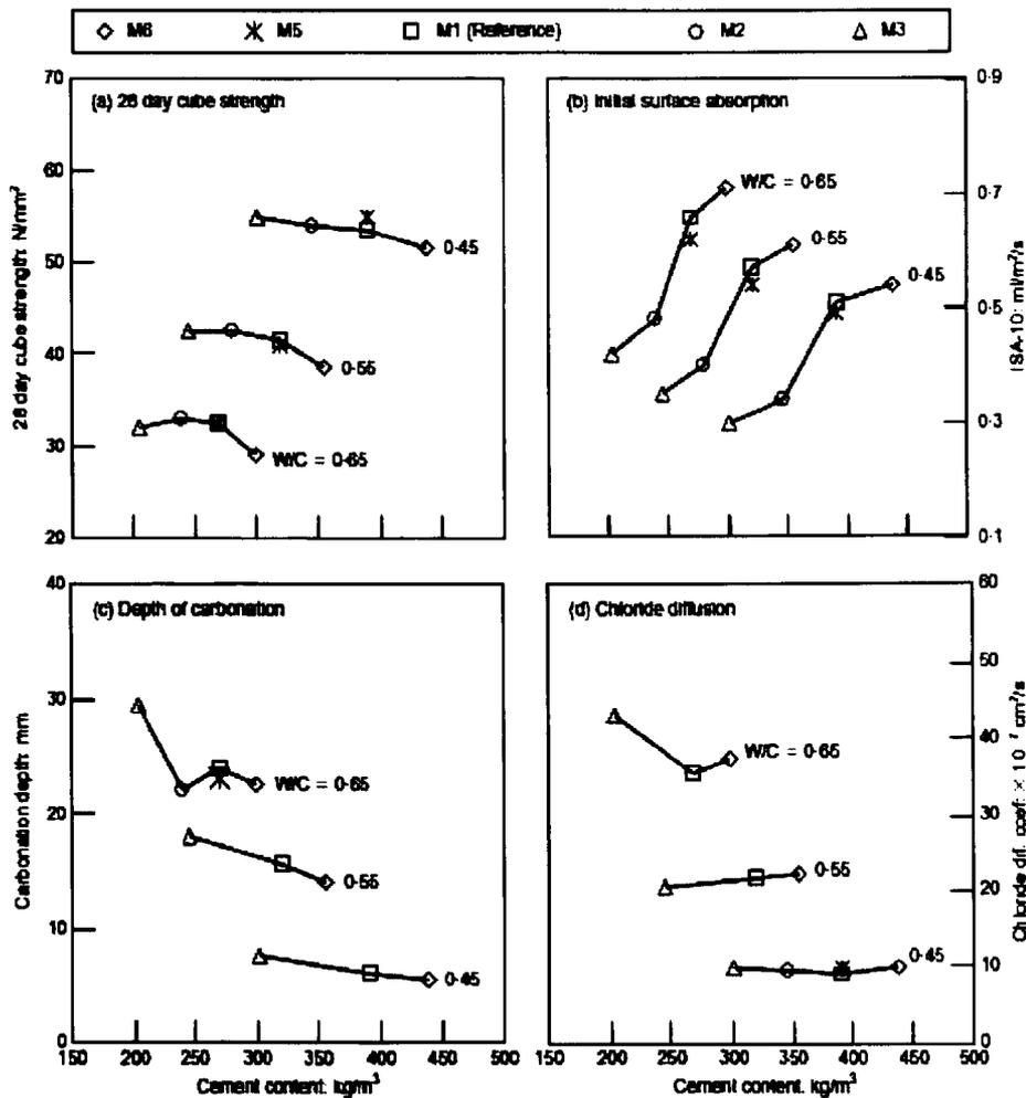
Figure 2-13 Influence of cement content on properties of PC concrete Dhir et al (2004)
