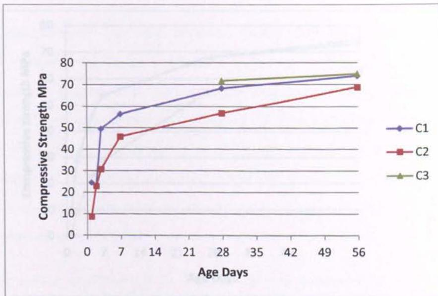
Figure 4-3 Compressive strength development of 70PC/30GGBS concrete mix
