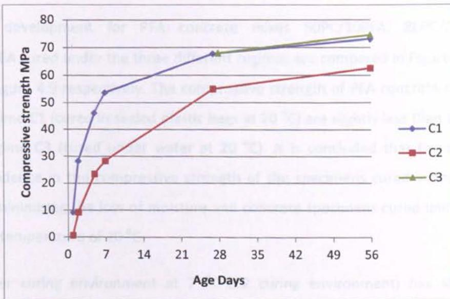
Figure 4-5 Compressive strength development of 50PC/50GGBS concrete mix
