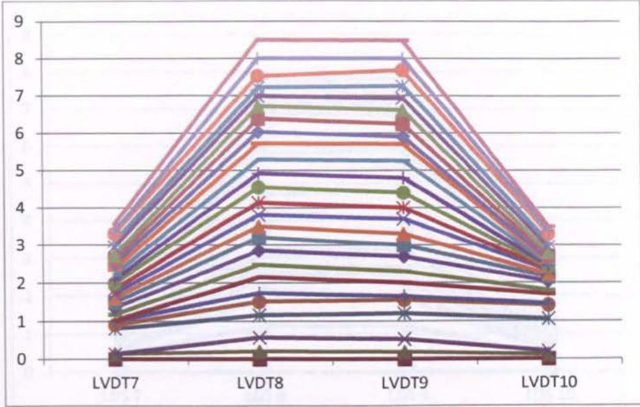
Figure C-7 Slab Deflection with support movement for 60PC/40GGBS
