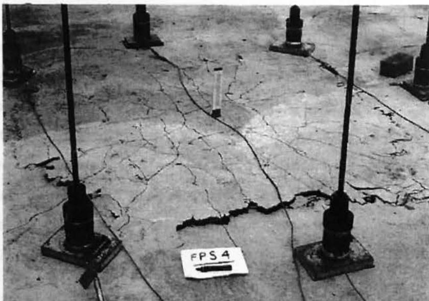
**Figure 2-20 Typical Failure Mode Chana & Desai (1992)**
