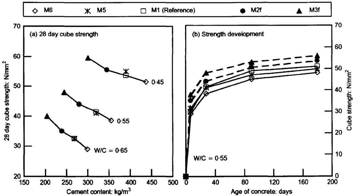
Figure 2-14 Influence of cement content on: (a) 28 day cube strength; (b) strength development of PC concrete Dhir et al (2004)
