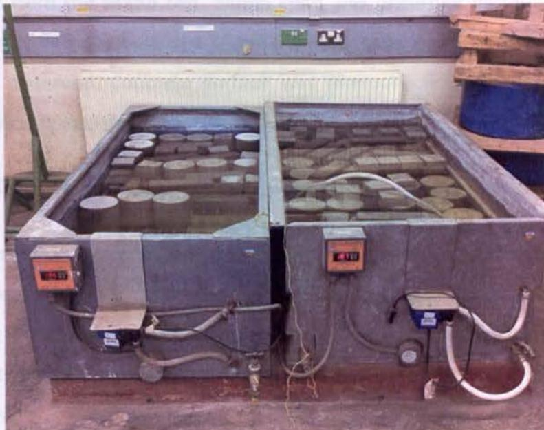
**Figure 3-7 Water curing environment (C3)**
