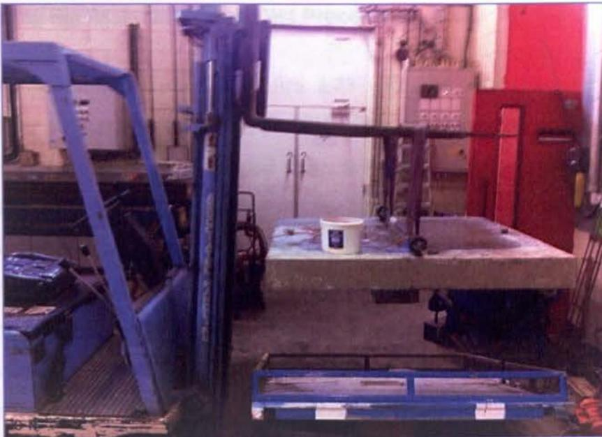
**Figure 3-21 Demoulding of slab specimen**
