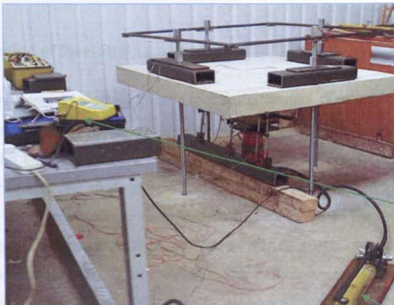
**Figure 3-14 Set up for punching shear strength test of flat slabs**
