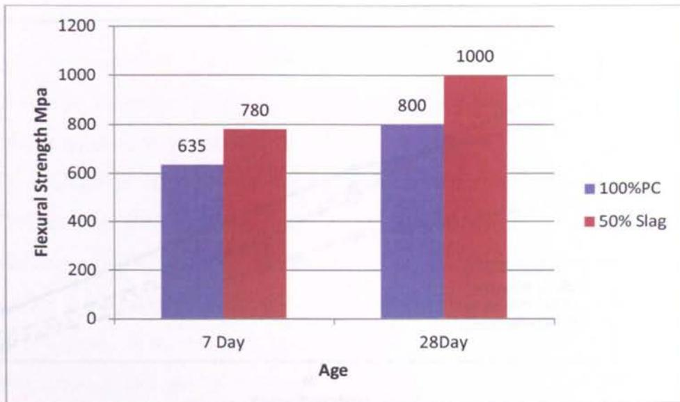
Figure 2-5 Effect of Slag on Flexural Strength of slag cement concrete after (SCA 2003)
