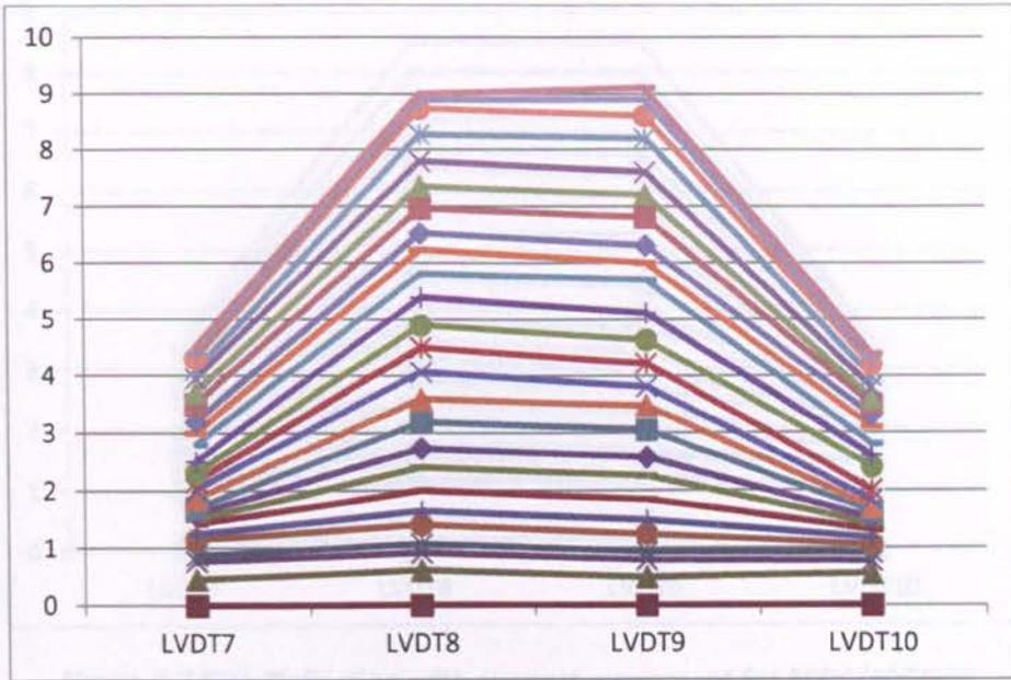
Figure C-5 Slab deflection with support movement for 70PC/30PFA
