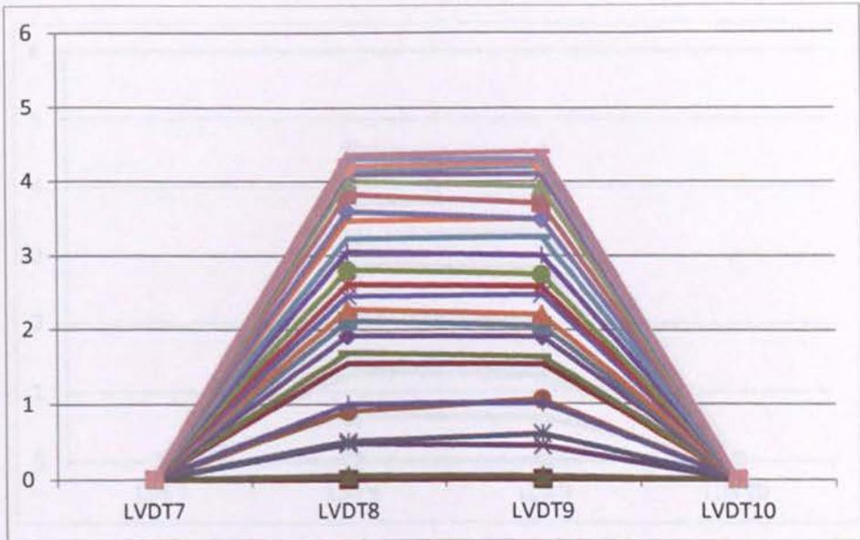
Figure C-8 Corrected Slab deflection for 60PC/40GGBS
