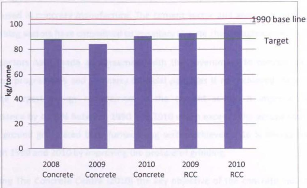
Figure 2-2 CO<sub>2</sub> emissions for production of concrete After (The Concrete Centre 2010)
