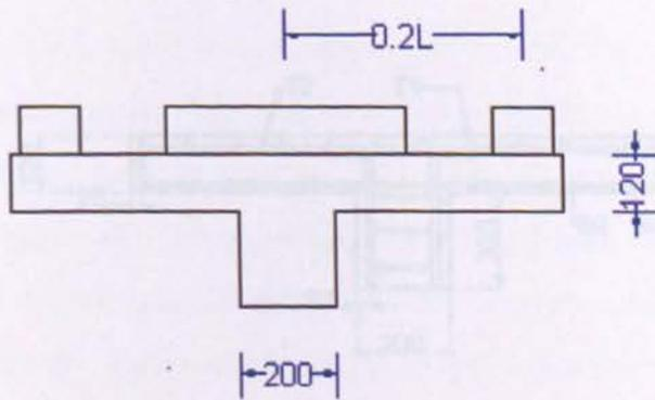
Figure 5-1 Specimen for Punching shear strength test
