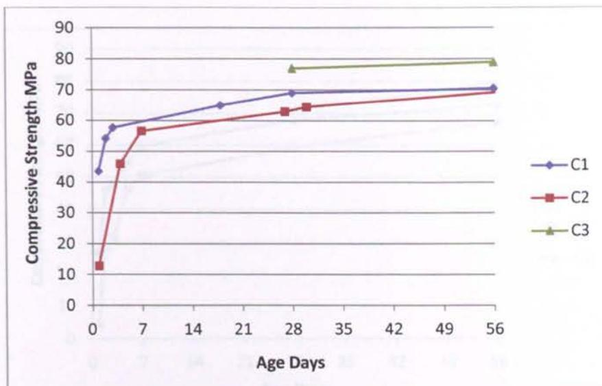
Figure 4-6 Compressive strength development of 100PC-Control concrete mix
