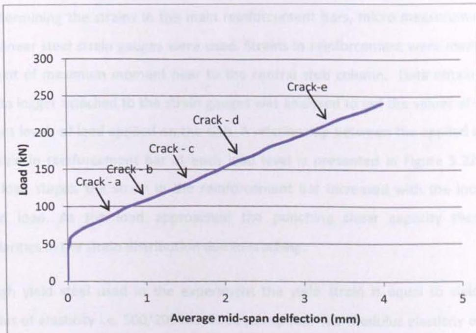
Figure 5-20 Average mid span deflection of 100PC-Control
