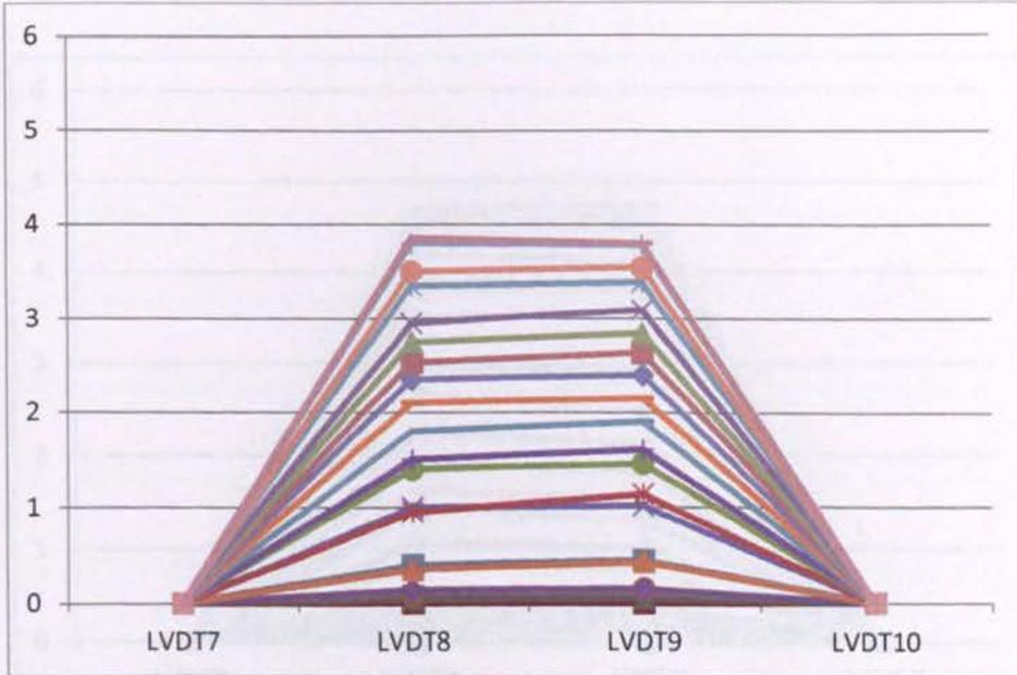
Figure C-4 Corrected slab deflection for 80PC/20PFA
