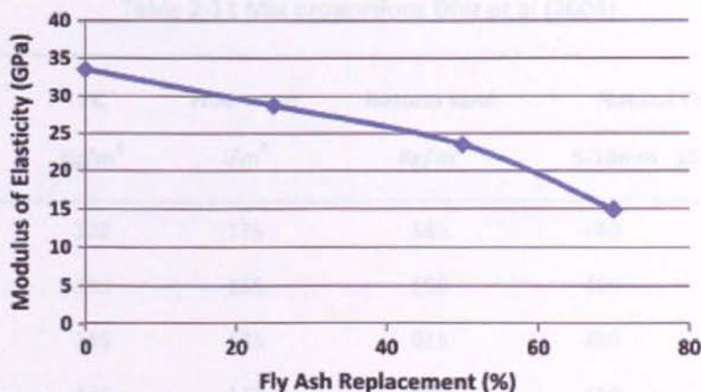
Figure 2-12 Trend of elastic modulus variation for Fly ash concrete (Kayali and Ahmed 2013)
