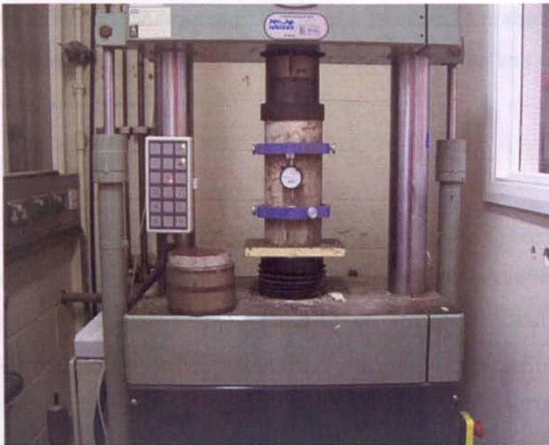
**Figure 3-11 Modulus of elasticity test**
