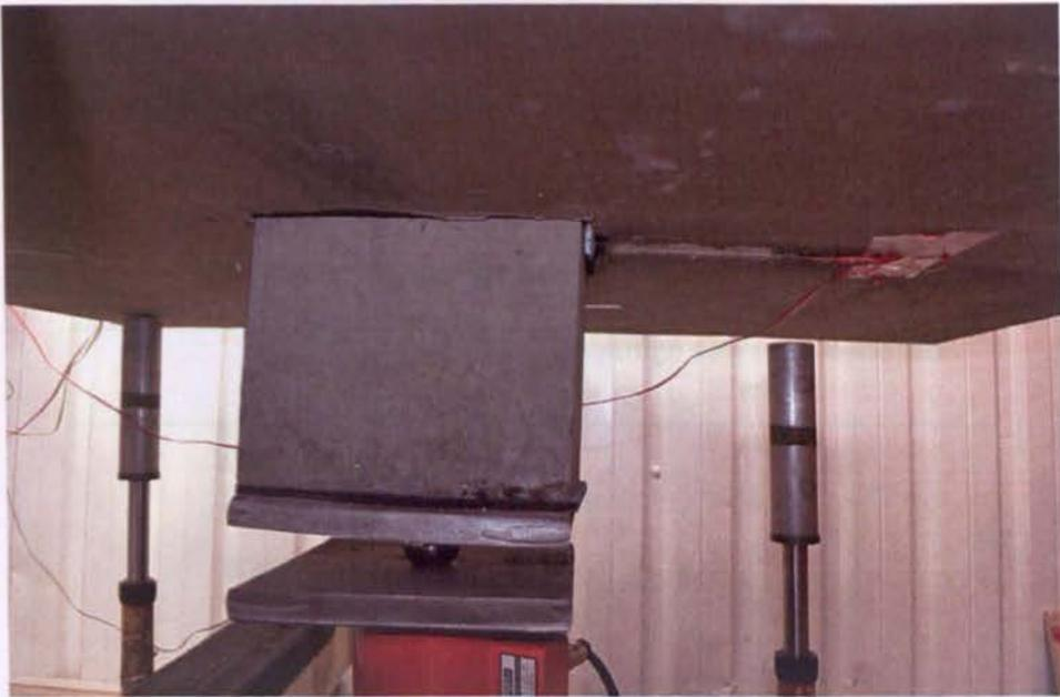
**Figure 5-12 80PC/20PFA Punched column in the slab after failure**
