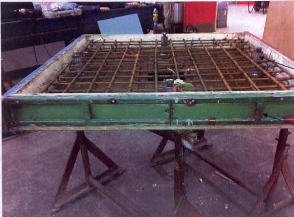
Insert with collar for making hole in the slab
