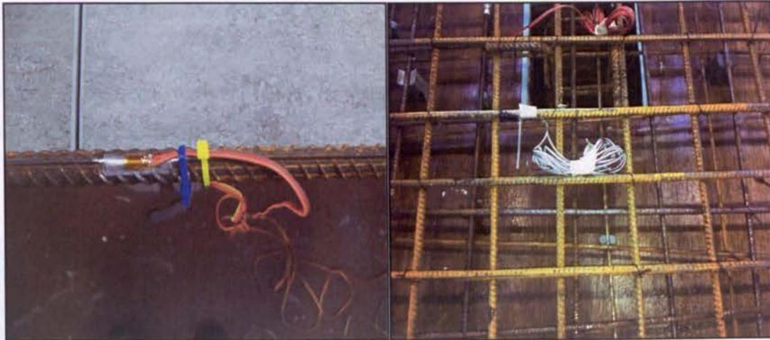
**Figure 3-16 Steel Strain Gauges**
