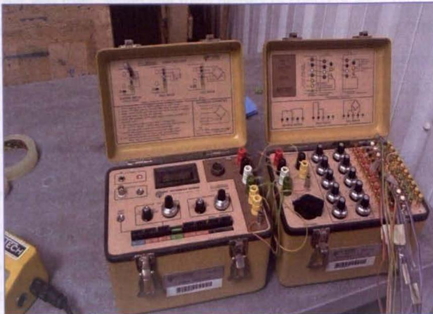
Figure 3-25 Data logger for strain gauges and LVDT's
