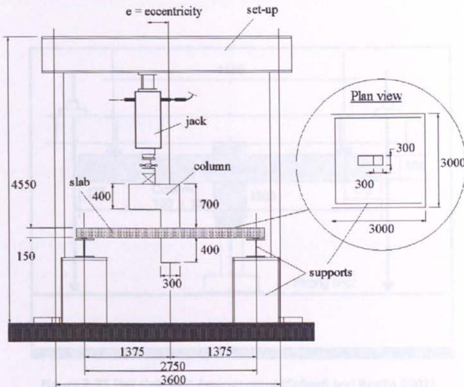
Figure 2-24 Testing a concrete flat slab specimen (Kruger, Burder & Favre 1998)
