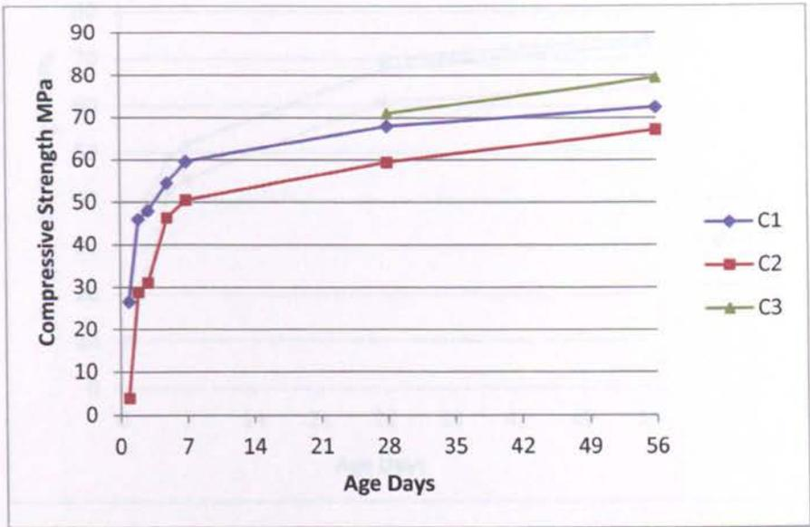
Figure 4-7 Compressive strength development of 90PC/10PFA concrete mix
