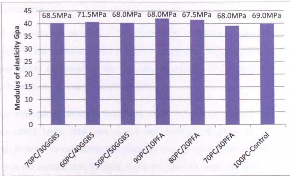
**Figure 4-17** Modulus of elasticity and compressive cube strength
