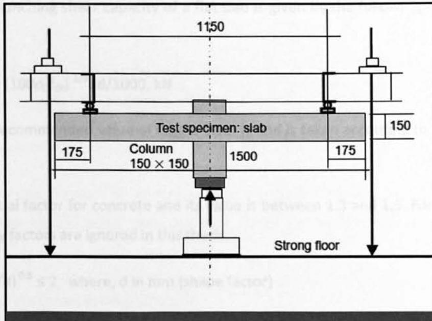
Figure 2-25 Flat slab Test Arrangement (Subedi and Baglin 2002)
