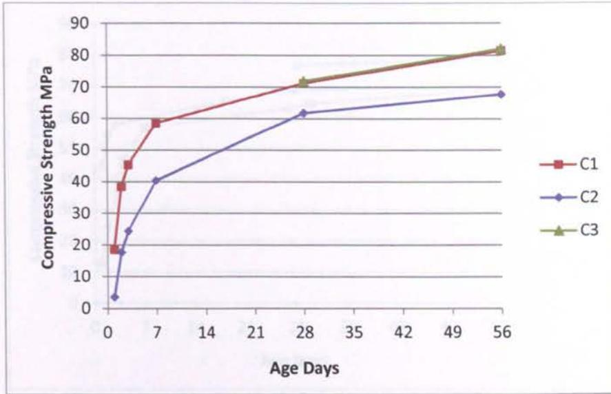
Figure 4-4 Compressive strength development of 60PC/40GGBS concrete mix
