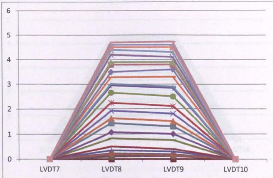
Figure C-6 Corrected Slab deflection for 70PC/30PFA
