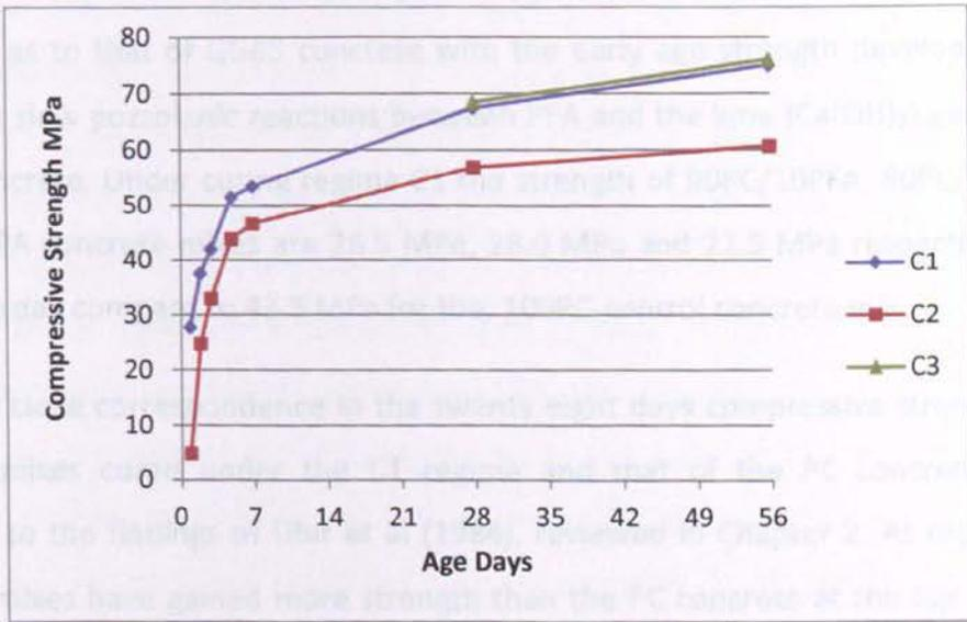
Figure 4-8 Compressive strength development of 80PC/20PFA concrete mix
