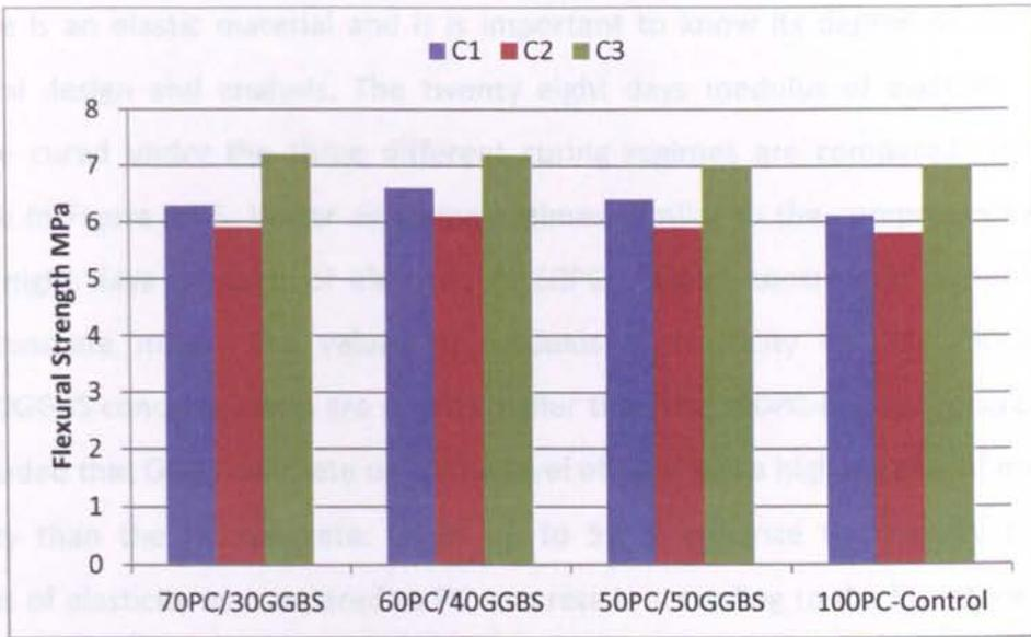
Figure 4-13 Flexural strength of GGBS concrete at the age of 28 days
