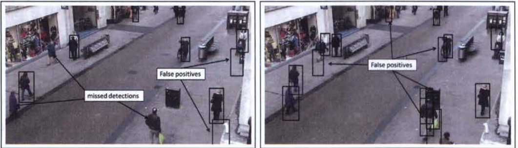
Figure 3.4: Sample detection results given by the HOG detector [30].
